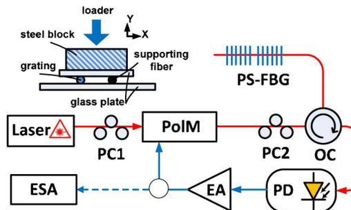
Fig. 1. Configuration of the proposed transverse load sensor. PolM, polarization modulator; PC, polarization controller; PD, photodetector; EA, electrical amplifier; ESA, electrical spectrum analyzer; PS-FBG, phase-shifted fiber Bragg grating; OC, optical circulator.
