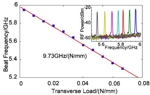
Fig. 4. Measured beating frequency as a function of applied transverse load and the electrical spectrum with different load. Inset: the electrical spectrum with different load.
