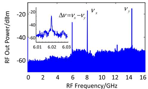
Fig. 3. Electrical spectrum of the signal generated by the dual-frequency OEO, with two microwave signals at 8.22 and 14.24 GHz and a beat signal at 6.02 GHz. Inset: the zoom-in view of the beat signal.
