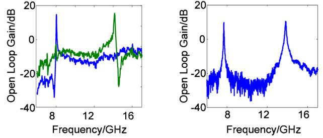
Fig. 2. (a) Single passband photonic microwave filter when the incident light is alighted with an angle of  $0^\circ$  or  $90^\circ$  relative to one principal axis of the PolM. (b) Dual passband photonic microwave filter when the incident light is alighted with an angle of  $45^\circ$  relative to one principal axis of the PolM.
