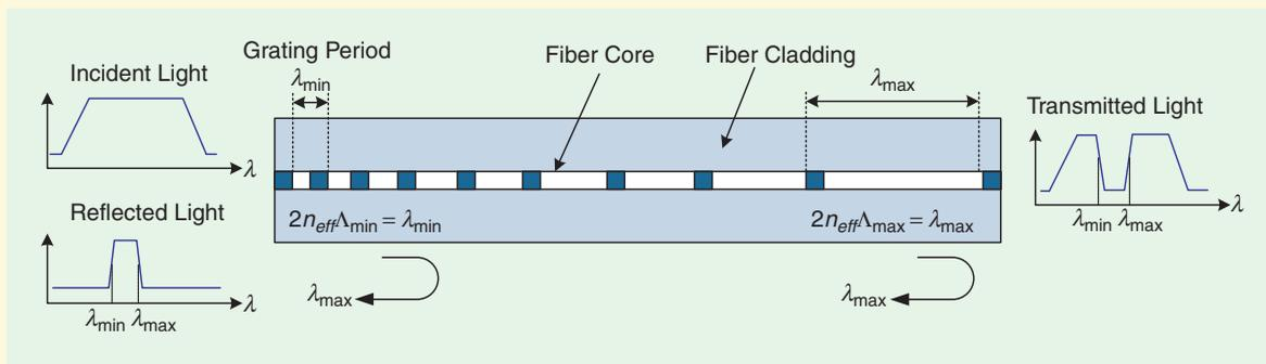
**Figure S2.** A chirped fiber Bragg grating.
