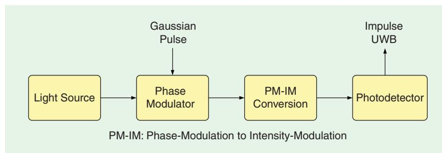
**Figure 4.** Ultrawideband pulse generation based on phase modulation and phase-modulation to intensity-modulation conversion.
