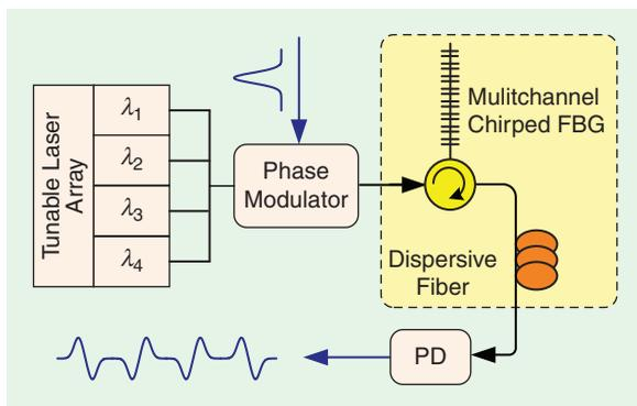
**Figure 15.** Ultrawideband coding using a multichannel fiber Bragg grating (from [22]).
