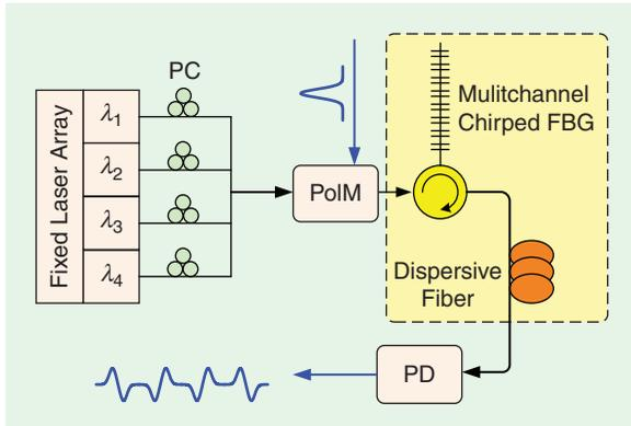
**Figure 18.** The ultrawideband phase-coding system, based on a polarization modulator with fixed optical wavelengths. PC: polarization controller. PolM: polarization modulator. PD: photodetector (from [22]).
