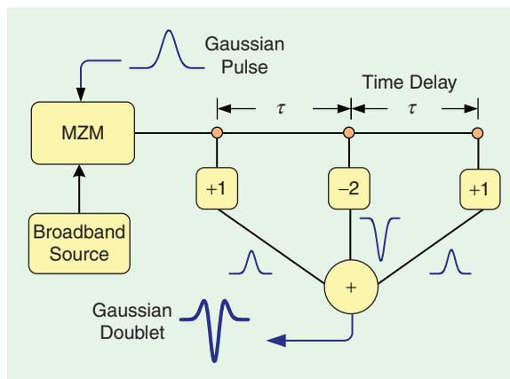
**Figure 11.** Ultrawideband doublet generation based on a three-tap photonic microwave delay-line filter with  $[1, -2, 1]$  as the three coefficients. MZM: Mach-Zehnder modulator.
