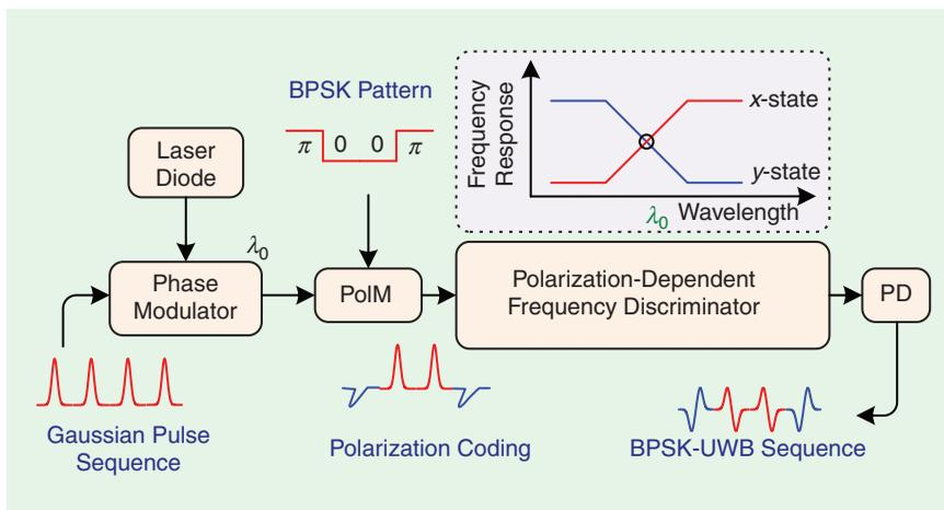
**Figure 19.** Generation of biphasic coding ultrawideband signals using a polarization modulator and a polarization-dependent frequency discriminator. Inset: The frequency response of the required polarization-dependent frequency discriminator. PolM: polarization modulator. PD: photodetector.
