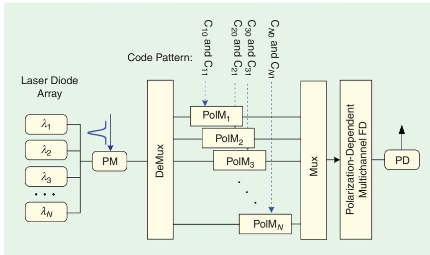
**Figure 24.** A multiuser ultrawideband-over-fiber system using a polarization modulator and a polarization-dependent multichannel frequency discriminator. PM: phase modulator. DeMux: demultiplexer. PolM: polarization modulator. Mux: multiplexer. PD: photodetector (from [23]).
