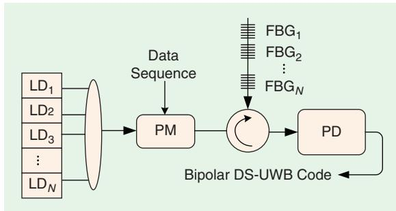
**Figure 14.** Bipolar ultrawideband coding using an array of fiber Bragg gratings. LD: laser diode. PD: photodetector.
