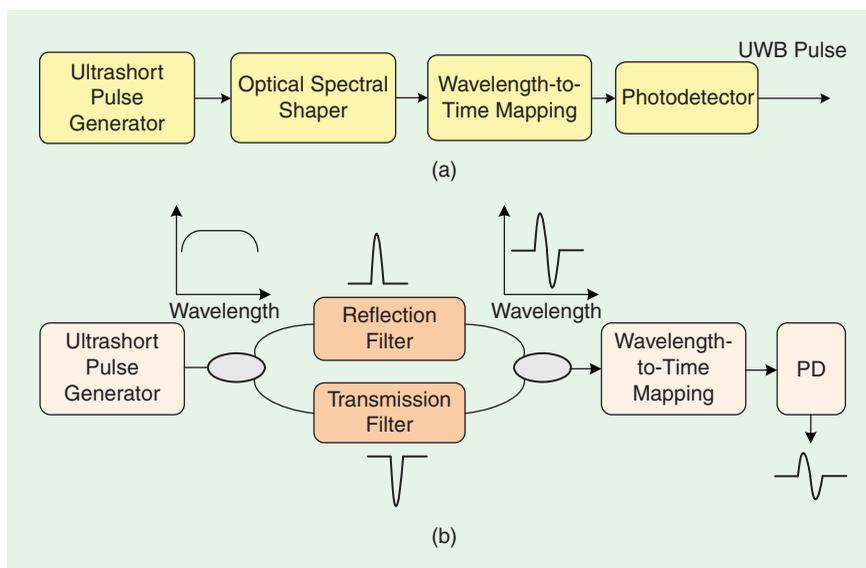
**Figure 13.** (a) Ultrawideband pulse generation based on spectral shaping and frequency-to-time mapping. (b) An all-fiber ultrawideband generation system. PD: photodetector.
