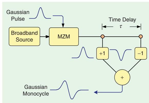
**Figure 8.** Ultrawideband monocycle generation based on a two-tap microwave delay-line filter with one negative coefficient. MZM: Mach-Zehnder modulator.
