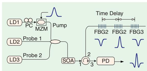
**Figure 12.** Ultrawideband doublet generation using a three-tap photonic microwave delay-line filter with one negative coefficient, generated using cross-gain modulation in a semiconductor optical amplifier. PC: polarization controller. SOA: semiconductor optical amplifier.
