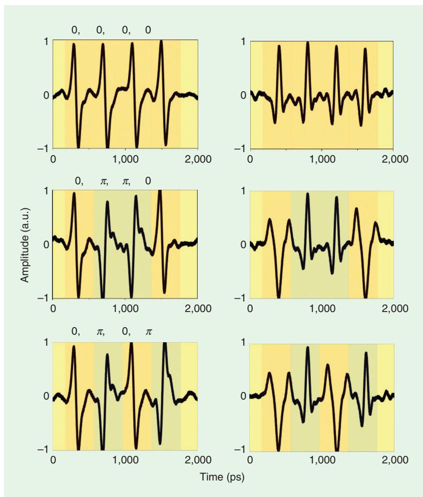
**Figure 17.** Phase-coded monocycle and doublet sequences corresponding to different code patterns measured in the time domain (from [22]).
