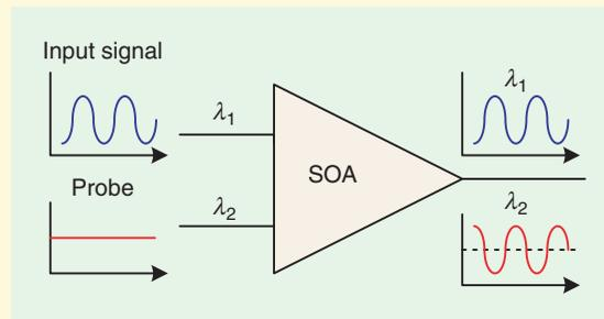
**Figure S3.** Cross gain modulation in a semiconductor optical amplifier (SOA). The input signal is carried by an optical carrier at a wavelength of  $\lambda_1$ . A continuous-wave optical probe at a wavelength of  $\lambda_2$  is sent to the semiconductor optical amplifier. At the output of the semiconductor optical amplifier, two complementary microwave signals carried by the optical carriers at  $\lambda_1$  and  $\lambda_2$  are obtained.
