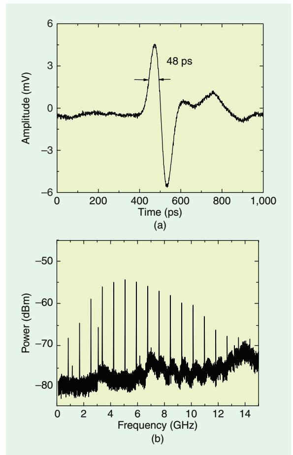
**Figure 10.** Ultrawideband monocycle pulse generated using a two-tap photonic microwave filter with one negative coefficient generated based on cross-gain modulation in a semiconductor optical amplifier; (a) the temporal waveform and (b) its spectrum.
