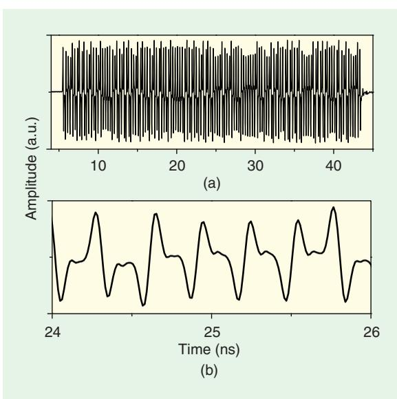
**Figure 21.** (a) The measured 127-chip binary phase-coded monocycle sequence and (b) a zoomed-in display (from [23]).
