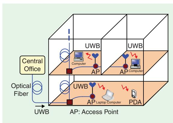
**Figure 2.** Ultrawideband-over-fiber system for broadband indoor wireless access (from [5]).
