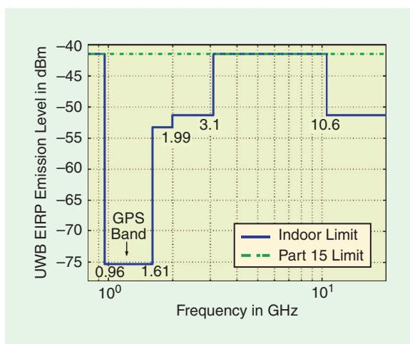
**Figure 1.** The ultrawideband frequency mask defined by the FCC for ultrawideband indoor communications (from [4]).
