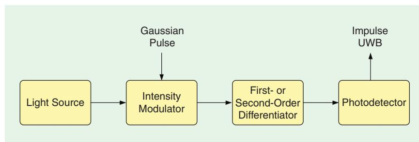
**Figure 3.** Generation of an ultrawideband monocycle or doublet pulse using a first- or second-order differentiator.
