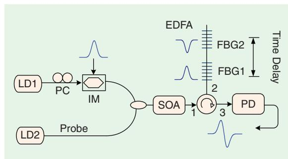
**Figure 9.** Ultrawideband monocycle generation based on a two-tap photonic microwave delay-line filter using a semiconductor optical amplifier. PC: polarization controller. IM: intensity modulator. EDFA: erbium-doped fiber amplifier. SOA: semiconductor optical amplifier.
