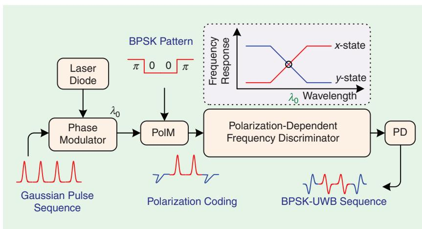
**Figure 19.** Generation of biphase coding ultrawideband signals using a polarization modulator and a polarization-dependent frequency discriminator. Inset: The frequency response of the required polarization-dependent frequency discriminator. PolM: polarization modulator. PD: photodetector.
