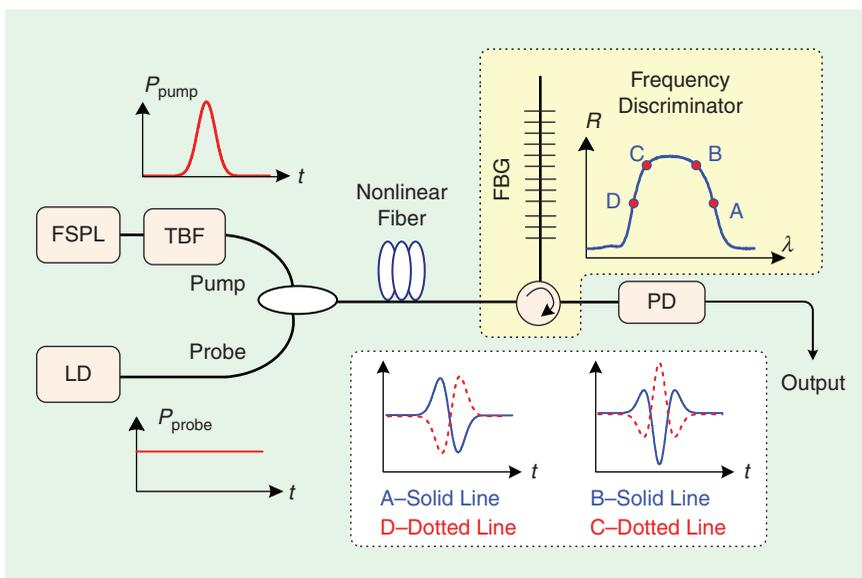
Figure 7. An all-optical ultrawideband pulse generator. The Gaussian pulse is generated by a femtosecond pulse laser with its spectrum sliced by a tunable bandpass filter to control the pulse width. Phase modulation is achieved in the 400-m dispersion-shifted fiber due to cross-phase modulation. LD: laser diode. PD: photodetector. FBG: fiber Bragg grating. FSPL: femtosecond pulsed laser. TBF: tunable bandpass filter.
