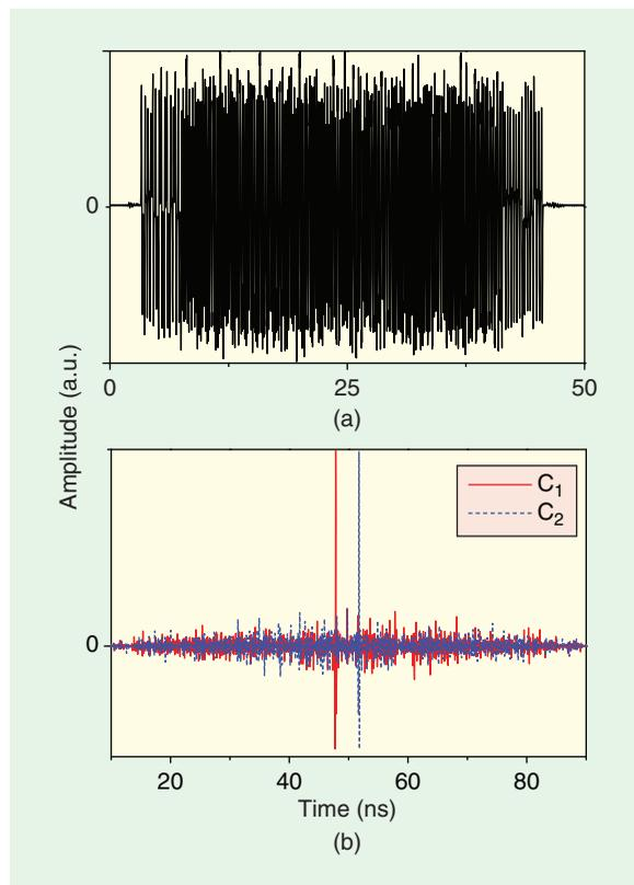
**Figure 25.** (a) The encoded output signal of a two-user ultrawideband-over-fiber system. (b) The signals are decoded by calculating the correlation between the measured encoding signal in (a) and the signature sequences corresponding to  $C_{11}$  and  $C_{21}$  (from [23]).
