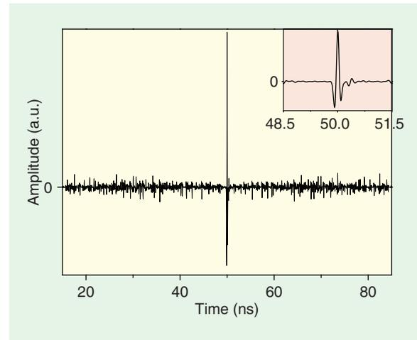
**Figure 22.** The signal is decoded by calculating the correlation between the measured signal and the signature sequence; the insert gives a zoom-in display of the correlation peak (from [23]).
