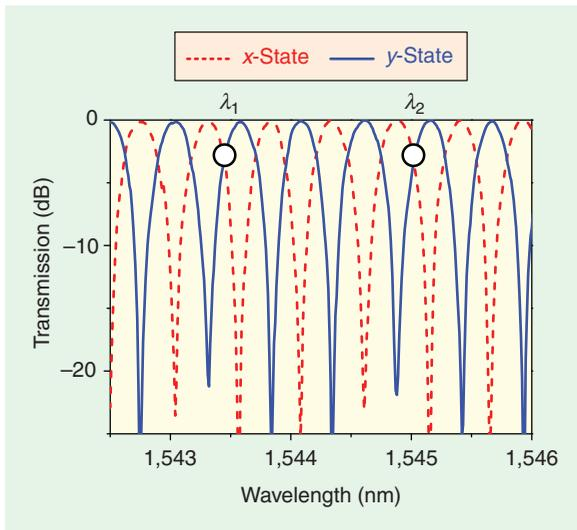
**Figure 20.** The transmission spectrum of a polarization-dependent frequency discriminator, consisting of a length of polarization-maintaining fiber and a polarizer (from [23]).
