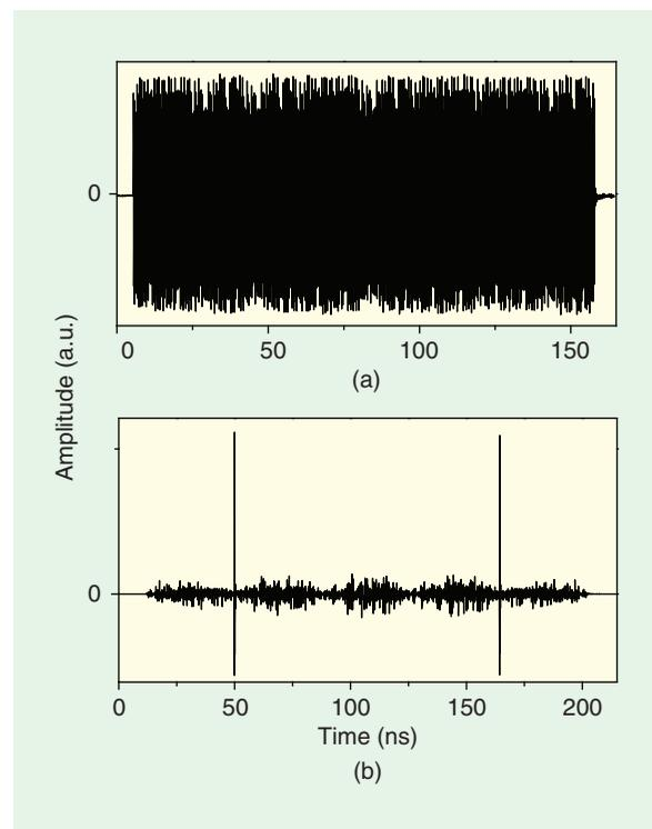
**Figure 23.** (a) The encoded signal when the code switch scheme is used. (b) The signal recovered by the correlator (from [23]).
