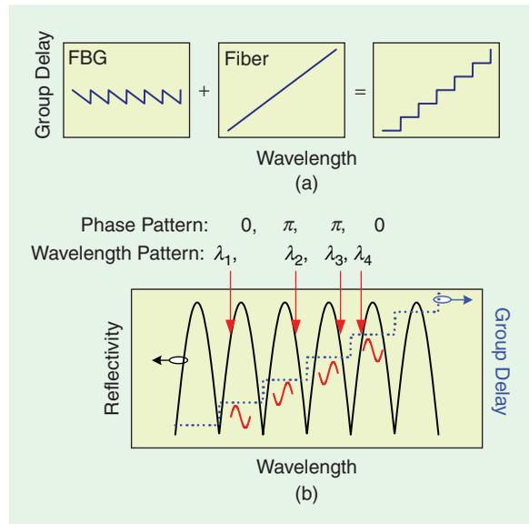
**Figure 16.** (a) Step-increasing group delay response generated by a multichannel chirped fiber Bragg grating in combination with a length of dispersive fiber. (b) Frequency response of the multichannel frequency discriminator (from [22]).
