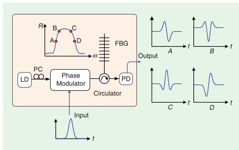
**Figure 6.** Experimental setup for ultrawideband pulse generation based on phase modulation and phase-modulation to intensity-modulation conversion.
