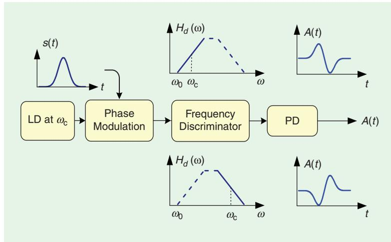
**Figure 5.** Gaussian monocycle pulse generation based on frequency discrimination.
