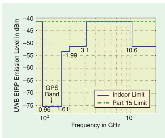
**Figure 1.** The ultrawideband frequency mask defined by the FCC for ultrawideband indoor communications (from [4]).
