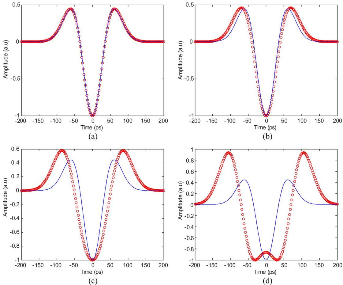
Fig. 7. Comparison of an ideal doublet and a doublet generated by using a microwave delay-line filter. Solid line: Ideal doublet. Circles: Doublet generated using the microwave delay-line filter. (a)  $\tau = 20$  ps. (b)  $\tau = 60$  ps. (c)  $\tau = 100$  ps. (d)  $\tau = 140$  ps.
