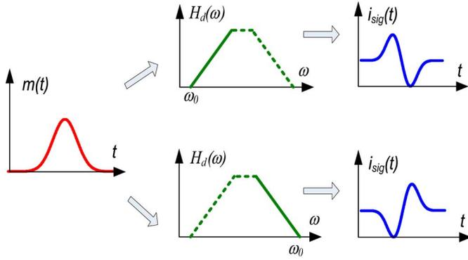
Fig. 2. UWB monocycle generation based on PM-to-IM conversion using an FBG-based frequency discriminator.
