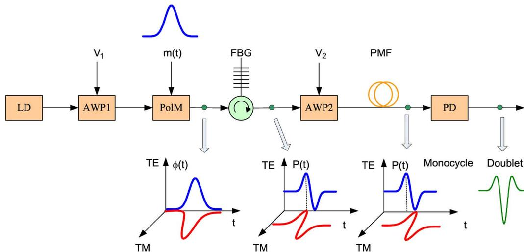
Fig. 1. Schematic of the electrically switchable UWB pulse generator. LD: Laser diode. AWP: Arbitrary wave plate. PolM: Polarization modulator. FBG: Fiber Bragg grating. PMF: Polarization Maintaining fiber. PD: Photodetector.
