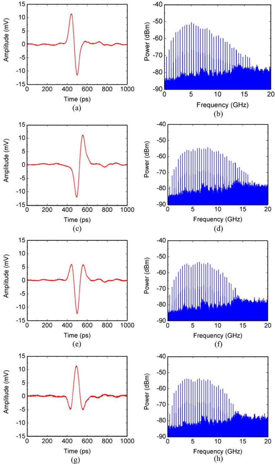
Fig. 5. Waveforms and spectra of the UWB Gaussian monocycle and doublet pulses generated in the experiment. Left column: Waveform. Right column: Spectrum. (a)–(d) Monocycles. (e)–(h) Doublets.
