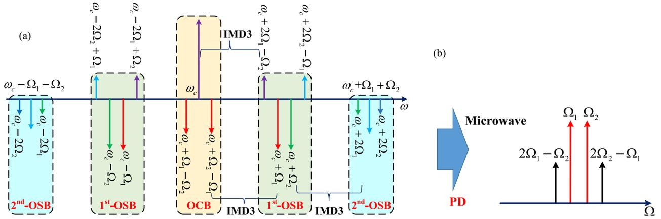
Fig. 2. Illustration of the generation of the IMD3 components of a conventional MPL, in which the MZM is biased at the quadrature point. (a) The optical spectral components at the output of the MZM, and (b) the spectrum of the detected electrical signal by the PD.
