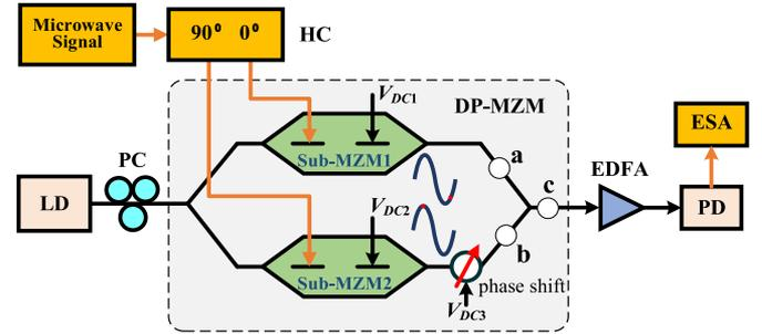
Fig. 1. Schematic diagram of the proposed MPL. HC: electrical  $90^\circ$  hybrid coupler, LD: laser diode, DP-MZM: dual parallel Mach-Zehnder modulator, PC: polarization controller, EDFA: erbium-doped fiber amplifier, PD: photodetector, ESA: electrical spectrum analyzer.
