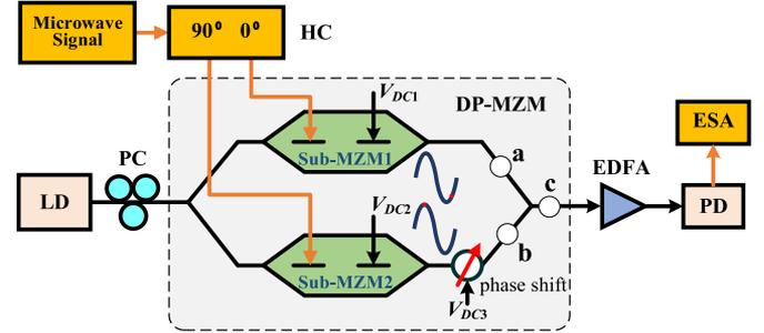
Fig. 1. Schematic diagram of the proposed MPL. HC: electrical  $90^\circ$  hybrid coupler, LD: laser diode, DP-MZM: dual parallel Mach-Zehnder modulator, PC: polarization controller, EDFA: erbium-doped fiber amplifier, PD: photodetector, ESA: electrical spectrum analyzer.
