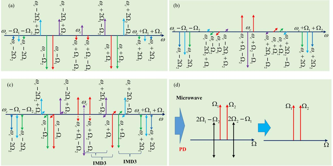
Fig. 3. The optical spectral components at (a) point a, (b) point b, and (c) point c in Fig. 1. (d) The recovered microwave signal at the output of the PD.
