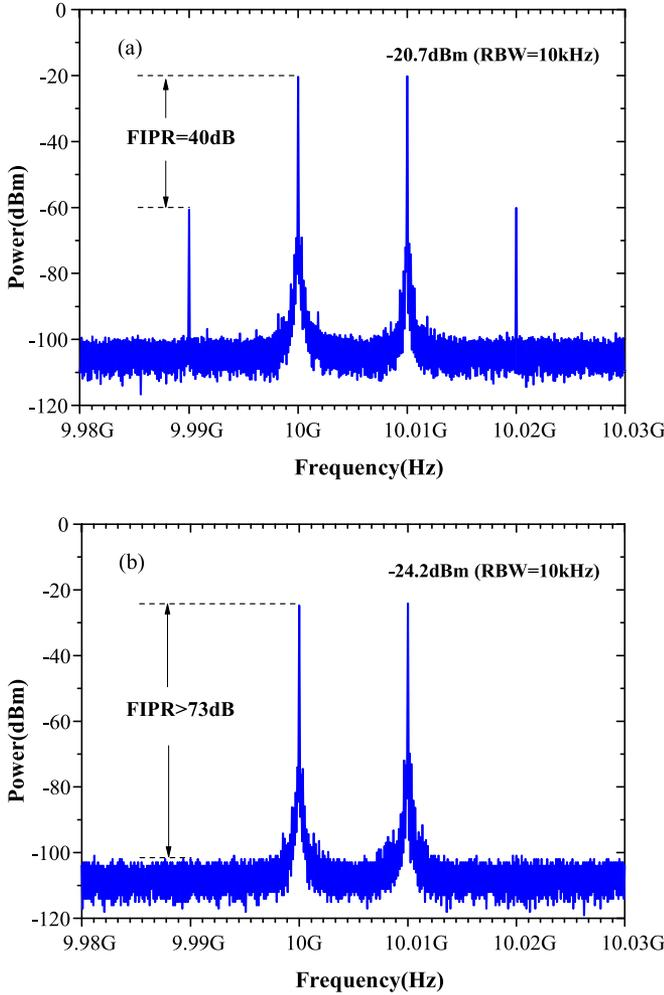
Fig. 5. Electrical spectrum of the microwave signal at the out of the PD. (a) A conventional IMDD link without IMD3 suppression, and (b) the proposed IMDD link with IMD3 suppression.
