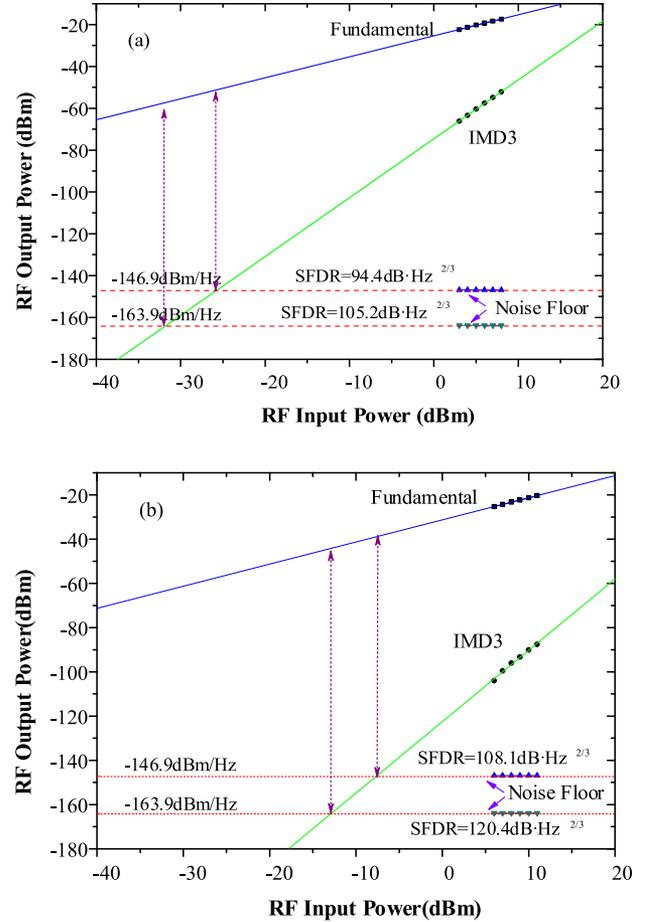
Fig. 6. Measured SFDR of the MPLs with and without IMD3 suppression. (a) Conventional IMDD MPL without IMD3 suppression, and (b) the proposed MPL with IMD3 suppression.
