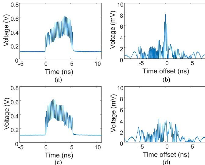
Fig. 6. (a) The PCMW generated at the output of PD2 with the TRM connected. (b) The signal at the output of PD1 with the signal in (a) as the input to the MPF. (c) The PCMW at the output of PD2 with the TRM disconnected. (d) The signal at the output of PD1 with the signal in (c) as the input to the MPF.
