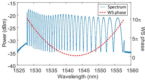
Fig. 2. The spectrum of the optical carrier measured at the output of the MZI when a quadratic phase is applied to the WS.
