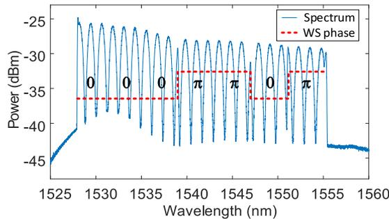
Fig. 5. The spectrum of the optical carrier measured at the output of the MZI when a 7-bit binary phase code is applied to the WS.
