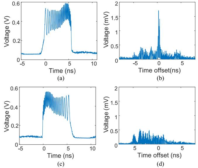
Fig. 4. (a) The LCMW generated at the output of PD2 with the TRM connected. (b) The signal at the output of PD1 with the signal in (a) as the input signal to the MPF. (c) The LCMW at the output of PD2 with the TRM disconnected. (d) The signal at the output of PD1, with the signal in (c) as the input signal to the MPF.
