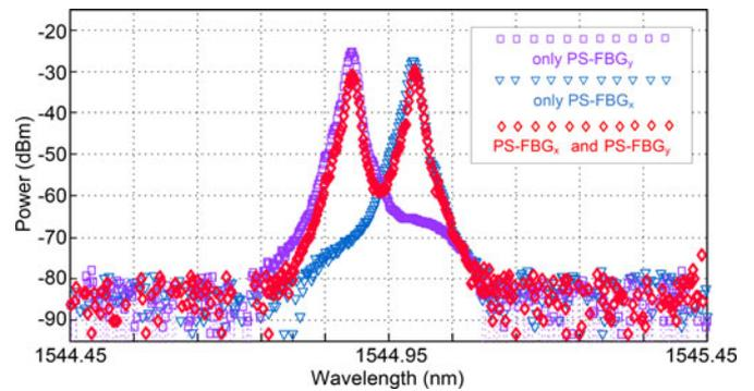
Fig. 6. Measured optical spectra of the output of the dual-wavelength fiber laser when it is configured at single wavelength and dual-wavelength operations.
