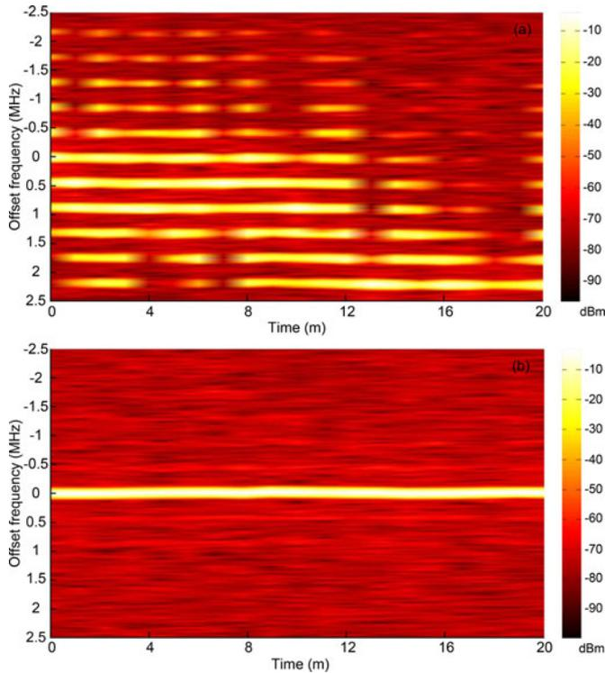
Fig. 7. The comparison of the generated microwave signal without and with the MIL. (span: 5 MHz; RBW: 4.7 kHz).
