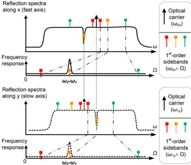
Fig. 3. The illustration of the formation of two equivalent MPBPFs. Upper: the MPBPF based on  $\omega_{2x}$  and PS-FBGy; lower: the MPBPF based on  $\omega_{1y}$  and PS-FBGx.
