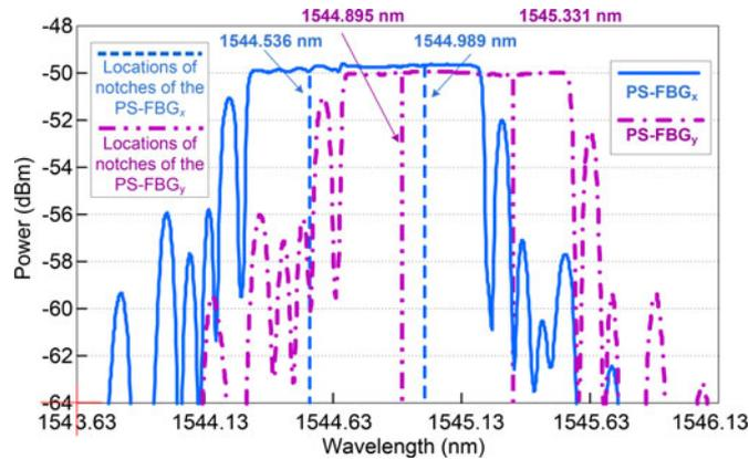
Fig. 5. Measured reflection spectral responses the PM-PS-FBG along its fast and the slow axis. (resolution: 0.01 nm).
