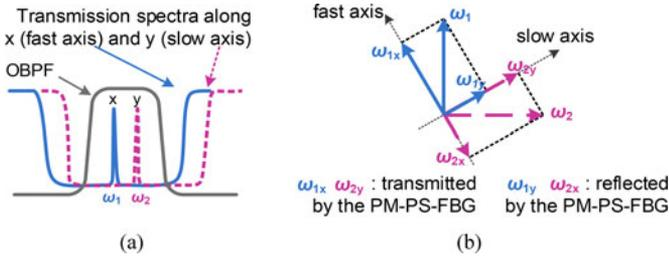
Fig. 2. (a) Transmission spectra of the OBPF and the PM-PS-FBG; (b) misalignment between the orthogonal polarization directions of  $\omega_1$  and  $\omega_2$  in the fiber laser and the fast and slow axes of the PM-PS-FBG.
