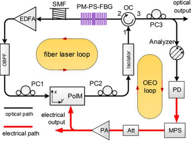
Fig. 1. Schematic of the mutually injection-locked OEO and DW-SLM fiber laser.
