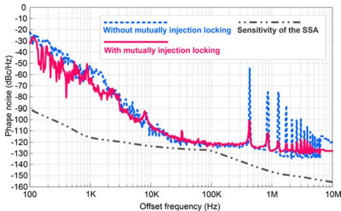
Fig. 8. Measured phase noise of the generated 11.8 GHz signal without (dashed line) and with (solid line) the MIL.
