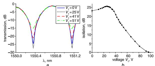
Fig. 2 Measured transmission spectra against different operation voltages applied to PMN-PT<sub>1</sub>, and channel isolation against applied voltage to PMN-PT<sub>1</sub>
