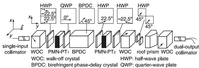
Fig. 1 Schematic of proposed tunable optical comb filter
