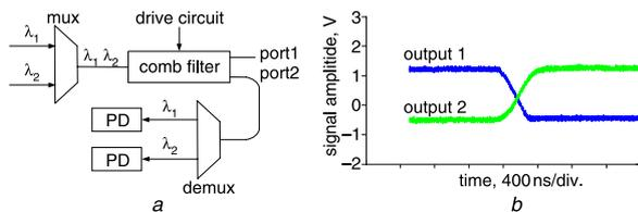
**Fig. 4** Experimental setup for evaluating tuning speed of comb filter and temporal response sampled from two PDs
