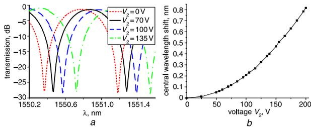
**Fig. 3** Measured transmission spectra for different voltages applied to PMN-PT<sub>2</sub>, and central wavelength shift against applied voltage  $V_2$
