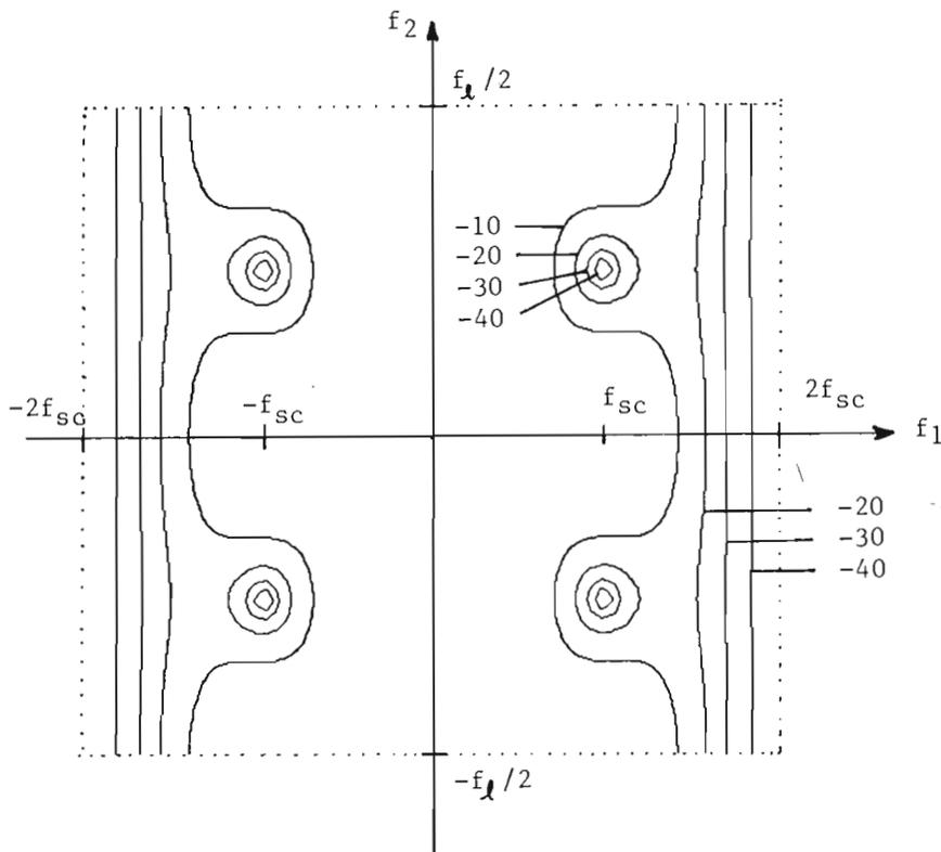
Figure 12. Frequency response of a filter of the type shown in Fig. 11. Attenuation in decibels shown on selected contours.
