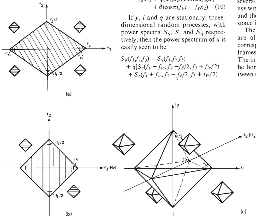
Figure 4. (a) Spatial projection of the basic spectrum of the NTSC color signal. (b) Vertical-temporal projection of the basic spectrum of the NTSC color signal. (c) Perspective view of the basic spectrum of the NTSC color signal.
