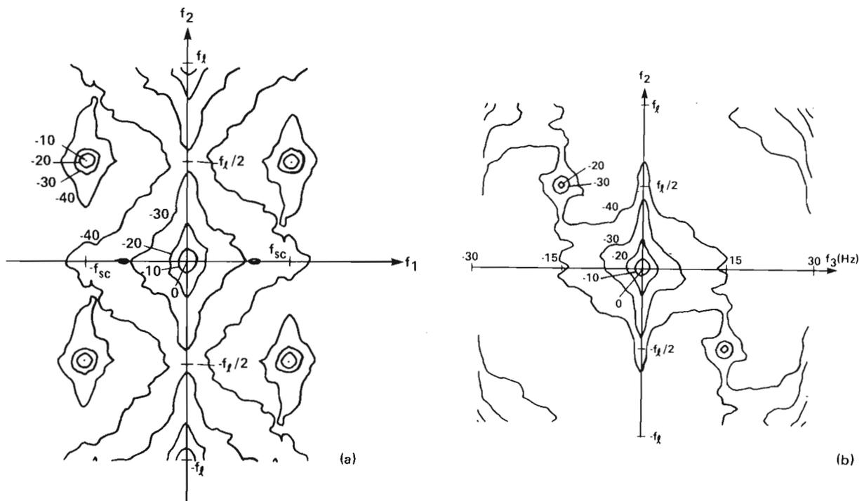
Figure 6. (a) Contours of spatial projection of measured spectrum for video signal sampled at  $4f_{sc}$ . (b) Contours of vertical-temporal projection of measured spectrum for video signal sampled at  $4f_{sc}$ . Relative power in decibels shown on selected contours.
