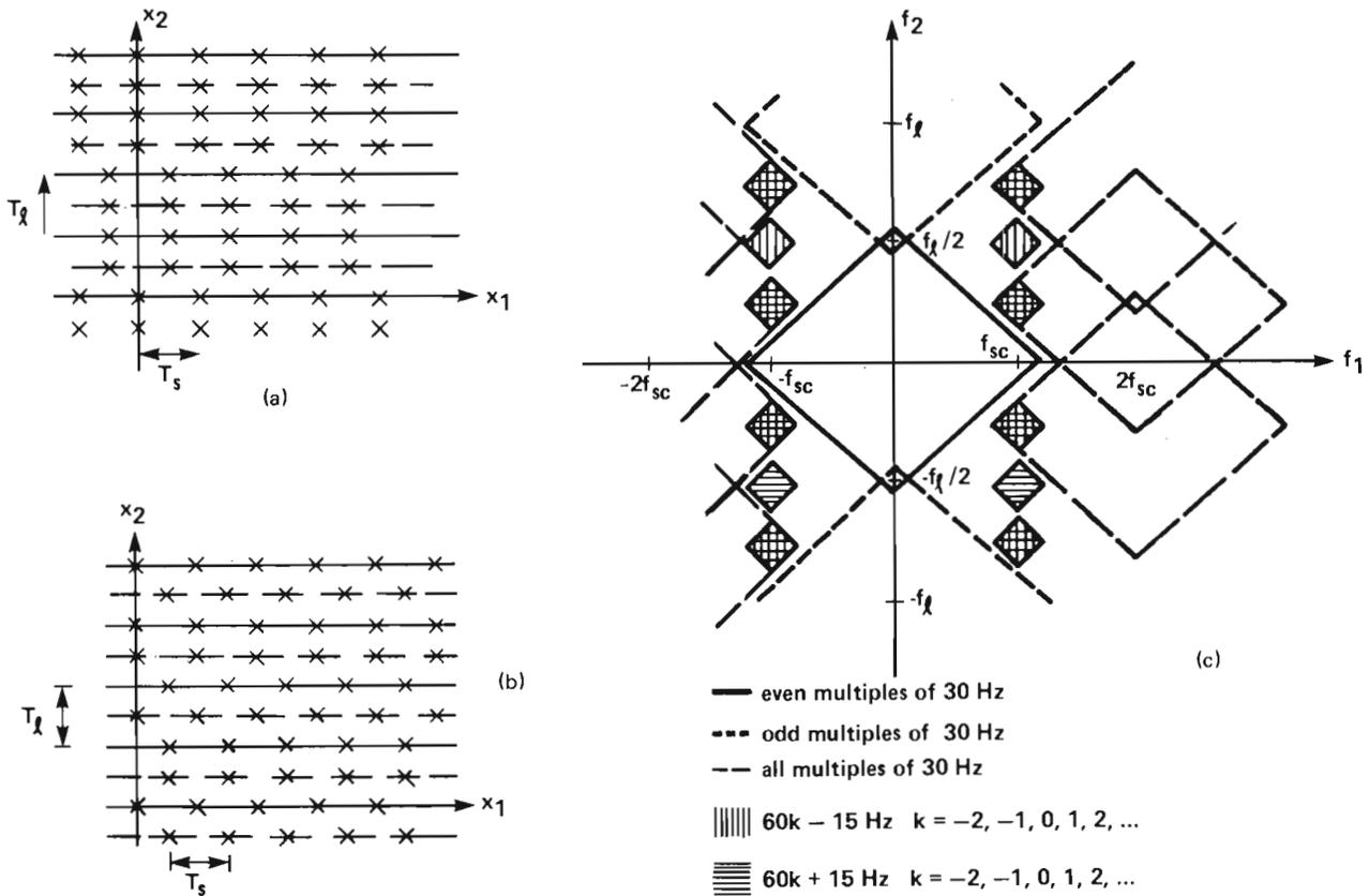
Figure 9. (a) Spatial projection of field-aligned double-checkerboard sampling pattern. (b) Spatial projection of field-offset double-checkerboard sampling pattern. (c) Spatial projection of spectrum of NTSC signal sampled at  $2f_{sc}$  with double-checkerboard sampling pattern.
