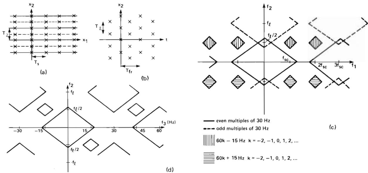
Figure 5. (a) Spatial projection of rectangular field-aligned sampling pattern. (b) Vertical-temporal projection of rectangular field-aligned sampling pattern. (c) Spatial projection of spectrum of NTSC signal sampled at  $3f_{sc}$  with rectangular field-aligned sampling pattern. (d) Vertical-temporal projection of spectrum of NTSC signal sampled with rectangular field-aligned sampling pattern.
