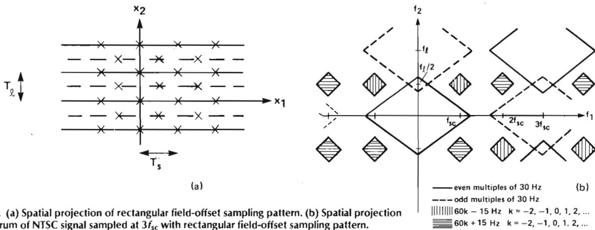
Figure 7. (a) Spatial projection of rectangular field-offset sampling pattern. (b) Spatial projection of spectrum of NTSC signal sampled at  $3f_{sc}$  with rectangular field-offset sampling pattern.
