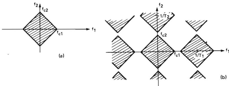
Figure 1. (a) Spatial projection of region of support for the spectrum of a three-dimensional function. (b) Spatial projection of spectrum of signal shown in (a), sampled with a rectangular sampling grid of period  $T_1$ ,  $T_2$ , and  $T_3$ .
