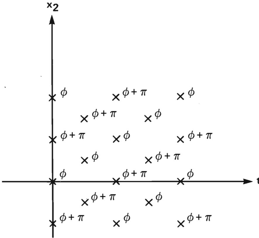
Figure 3. Subcarrier phase relationships for the NTSC color signal.
