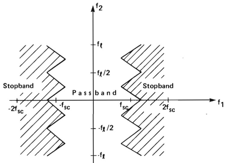
Figure 10. Pass-stop characteristic of ideal two-dimensional filter to reconstruct signal sampled with double-checkerboard sampling pattern.
