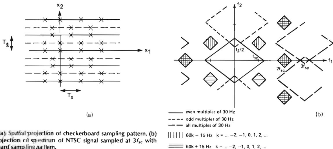
Figure 8. (a) Spatial projection of checkerboard sampling pattern. (b) Spatial projection of spectrum of NTSC signal sampled at  $3f_{sc}$  with checkerboard sampling pattern.
