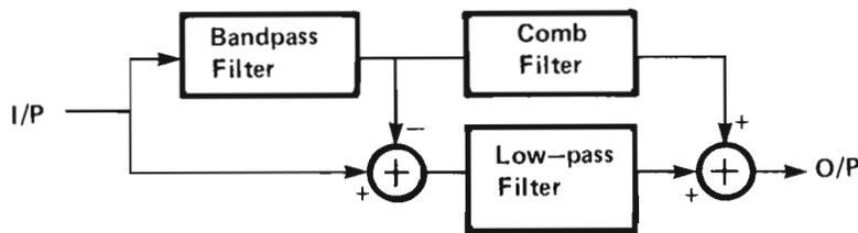
Figure 11. A possible filter structure to approximate the ideal characteristic of Fig. 10.
