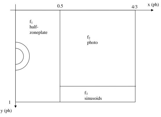
You should create three images A, B, C and mosaic them as Z=[A [B; C]]. Use meshgrid to generate A and C, of course making the appropriate adjustments to size, spacing, etc. Note that  $u_1, v_1, u_2, v_2$  have units of c/ph and r is in ph.
