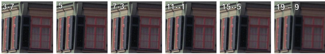
Figure 27: Alfred picture details for the transition band position of the anti-aliasing filter used for the  $1024 \times 1536$  image. The width is of  $10c/px$ .
