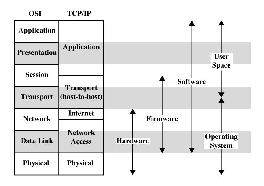
Figure 1.11 A Comparison of the TCP/IP and OSI Protocol Architectures
