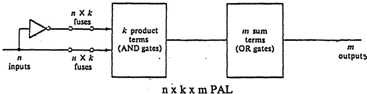
IMPLEMENTING AN  $n$ -INPUT,  $m$ -OUTPUT COMBINATIONAL CIRCUIT
