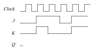
Q8. Find the input for a rising-edge T flip-flop which will produce the output Q as shown. Assume T begins at 0, and ignore propagation delays. (2)
