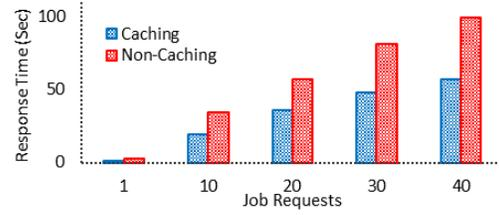
Fig.7. Average response time for file/block access with varying number of job requests.
