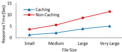
Fig.6. Average response time for file/block access with varying sizes.
