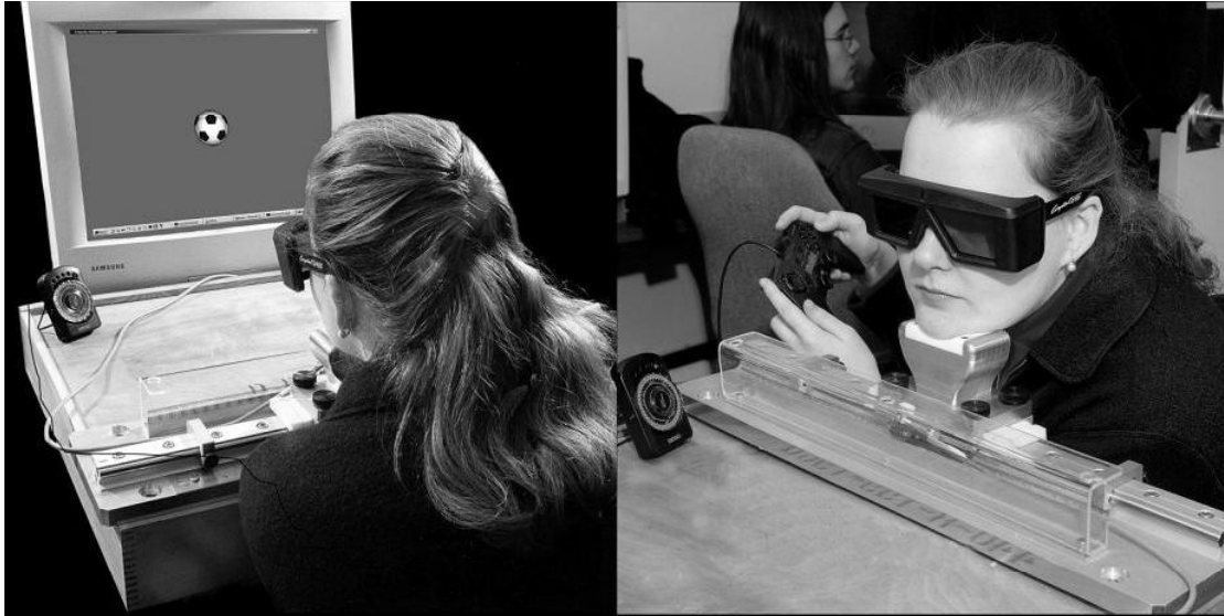
Figure 1. Apparatus used to monitor the head position of the viewer, display the stereoscopic images, and record the viewer's response.
