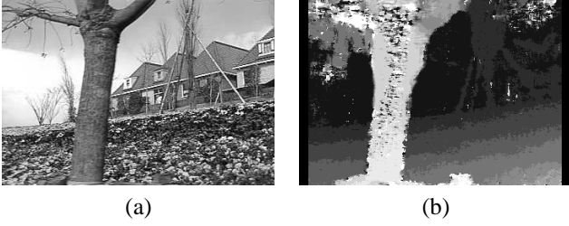
Fig. 2. (a) Original middle image of Flower Garden ; (b) the coarse disparity estimated by the phase method
