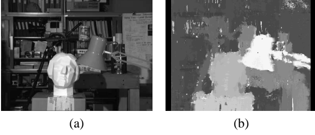
Fig. 1. (a) Original middle image of Tsukuba ; (b) the coarse disparity estimated by the phase method
