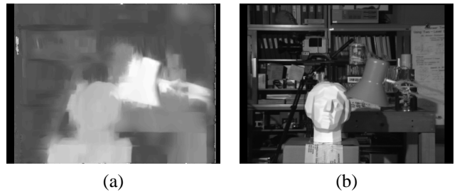
Fig. 3. (a) Refined disparity field for Tsukuba ; (b) interpolated middle image, 30.04dB
