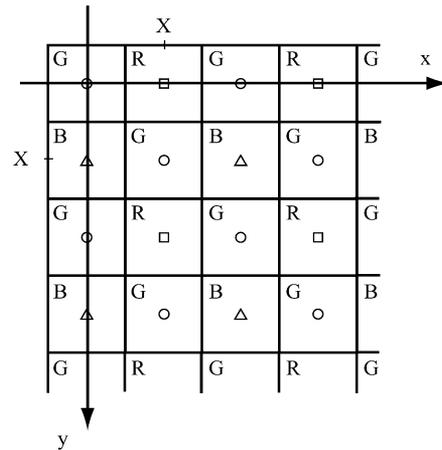
Fig. 1. Upper left portion of the Bayer CFA sampling structure, showing the constituent sampling structures  $\Lambda_R(\square)$ ,  $\Lambda_G(\circ)$ , and  $\Lambda_B(\triangle)$ .
