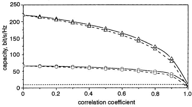
**Fig. 1** BLAST channel capacity against correlation coefficient,  $\rho = 30$  dB
