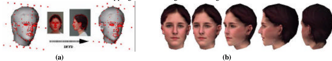
Figure 2: (a) Modification of a generic head according to feature points detected on pictures. Points on a 3D head are control points for DFFD. (b) Snapshots of a reconstructed head in several views.
