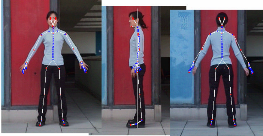
Figure 7-10: Automatic Skeleton fitting with feature points.
