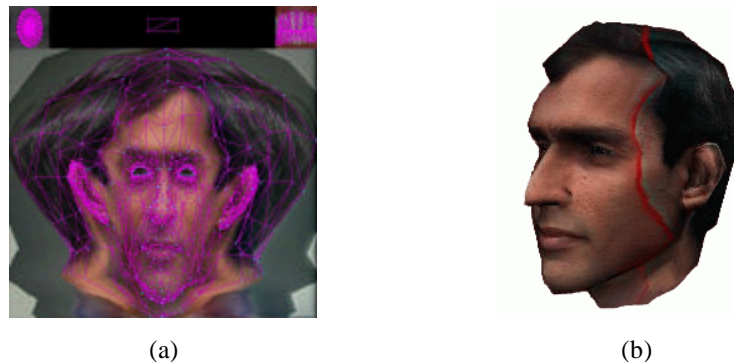
Figure 3-16: (a) Texture coordinates. (b) A textured head with curves on. The left part and the right part of the curves are the different sources of texture mapping.
