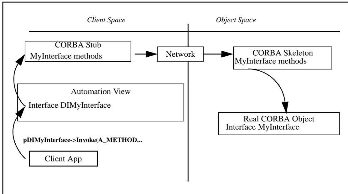
Figure 19-2 Methods of the Automation View Interface Delegate to the CORBA Stub
