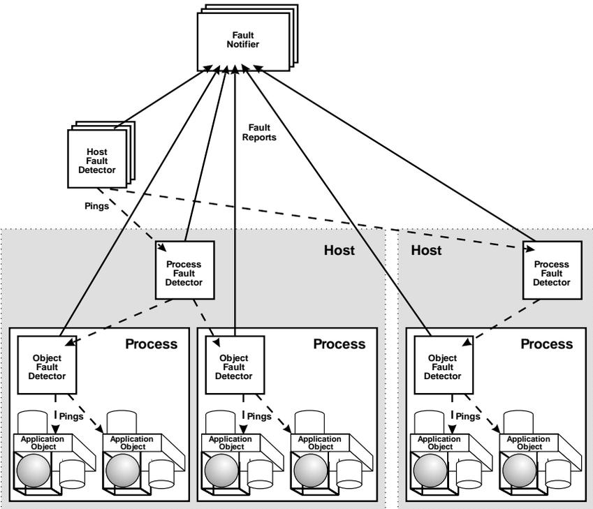
Figure 23-8 Hierarchical Fault Detection.
