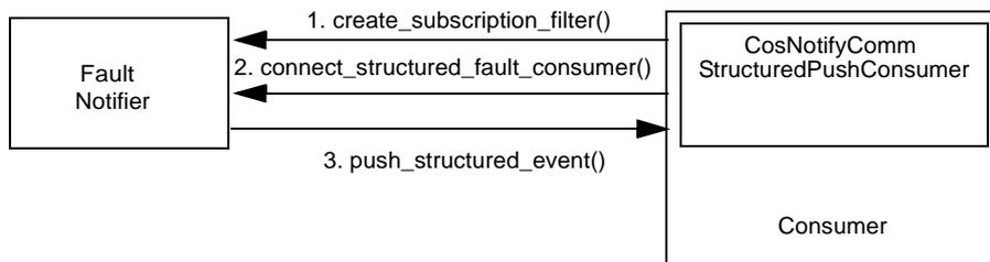
Figure 23-11 Connection Setup between the Consumer and the Fault Notifier
