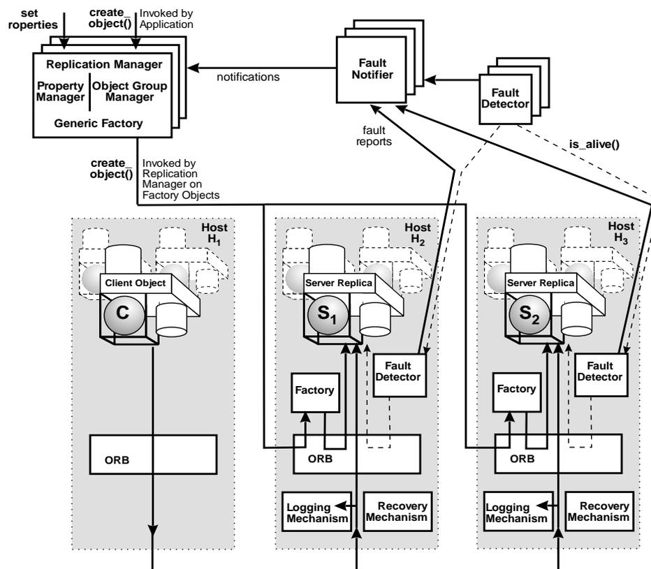
Figure 23-2 Architectural Overview of a Fault-Tolerant System
