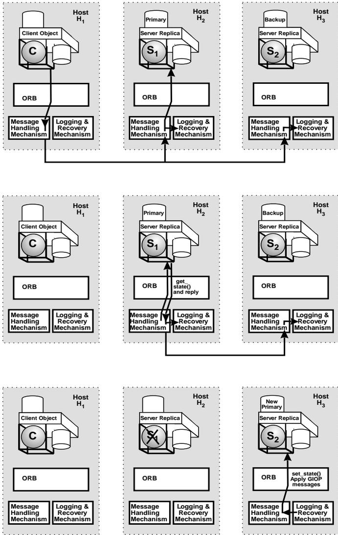
Figure 23-12 Operation of the Logging and Recovery Mechanisms for a server object group having the WARM\_PASSIVE ReplicationStyle, during normal operation, during the recording of a checkpoint, and during recovery
