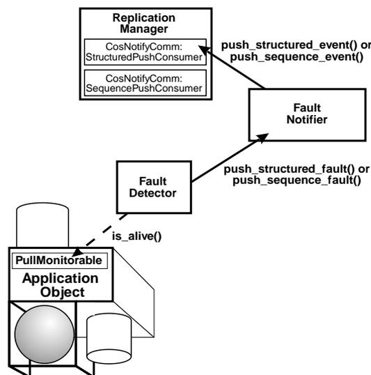
Figure 23-9 PULL FaultMonitoringStyle.
