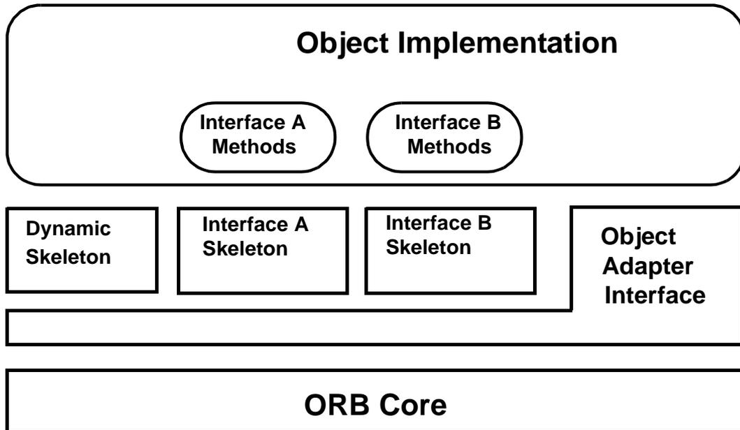
Figure 2-8 The Structure of a Typical Object Adapter
