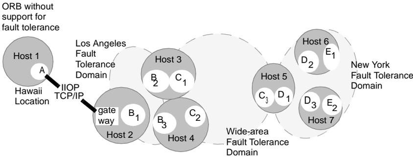
Figure 23-1 Fault tolerance domains are shown lightly shaded, hosts are shown darkly shaded, and members of an object group are shown unshaded. The members of object group B are denoted B<sub>1</sub>, B<sub>2</sub> and B<sub>3</sub>, and similarly for object groups C, D and E.
