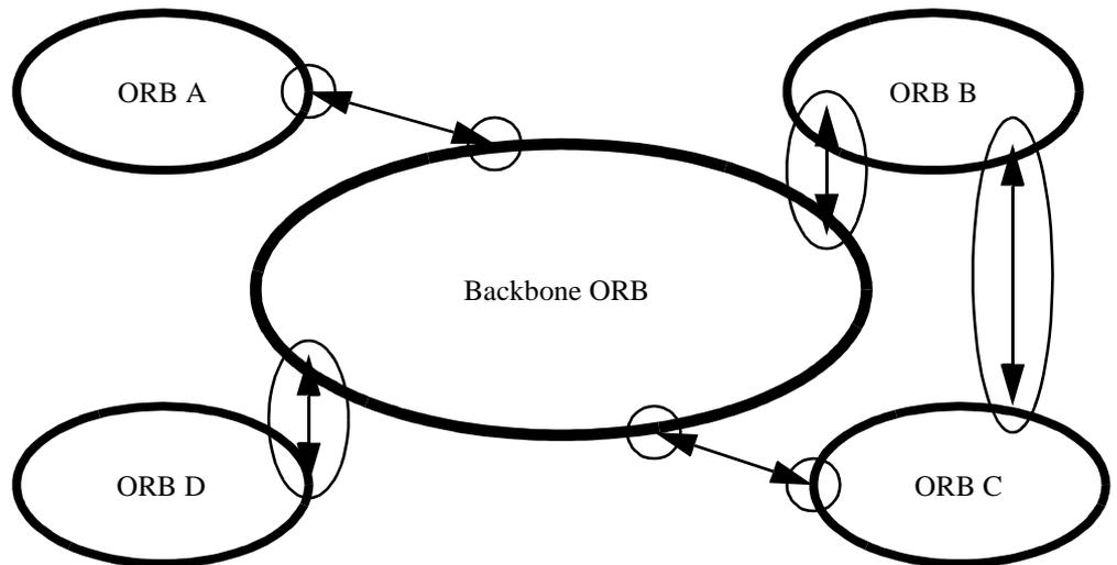
Figure 13-3 An ORB chosen as a backbone will connect other ORBs through bridges, both full-bridges and half-bridges.
