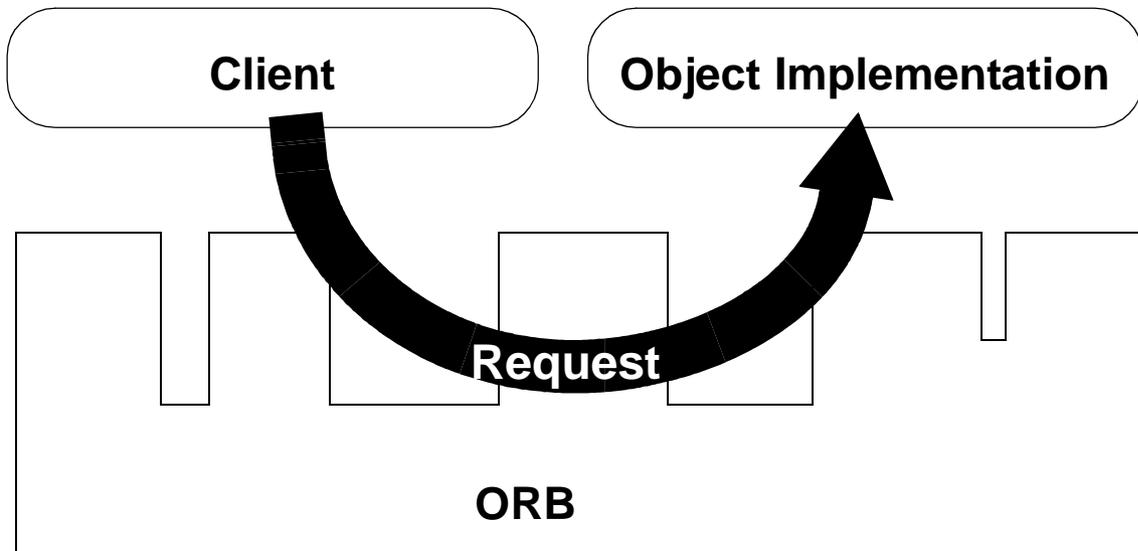
Figure 2-1 A Request Being Sent Through the Object Request Broker
