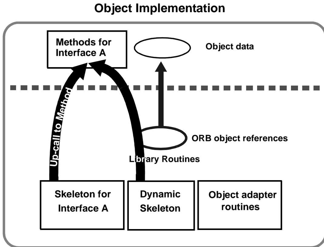
Figure 2-7 The Structure of a Typical Object Implementation
