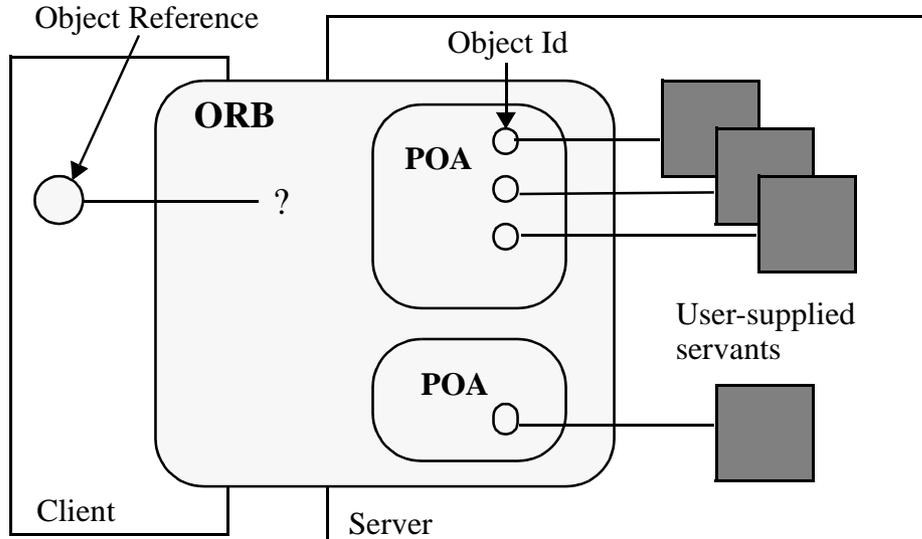
object not present in the Active Object Map, the POA either uses the default servant to perform the request or it invokes the servant manager to obtain a servant to perform the request. If the **RETAIN** policy is used, the servant returned by a servant manager is retained in the Active Object Map. Otherwise, the servant is used only to process the one request.
