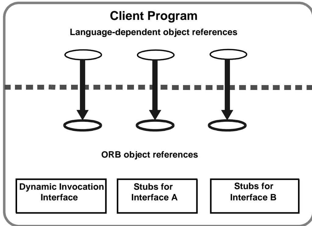
Figure 2-6 The Structure of a Typical Client
