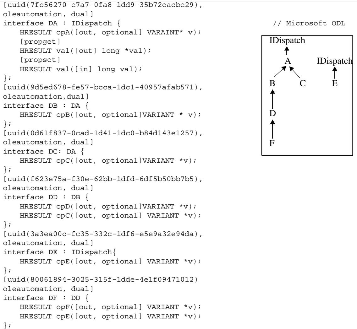
Figure 17-6 Example: ODL Mapping for Multiple Inheritance
