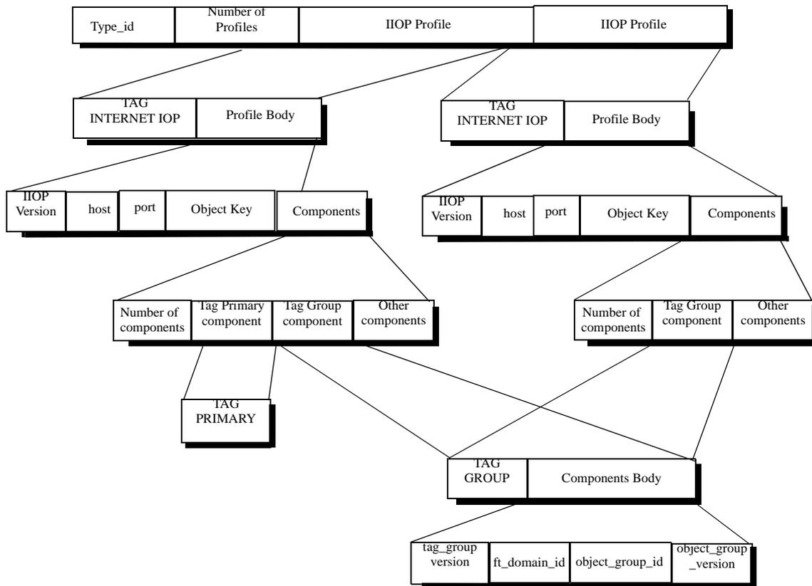
*Figure 23-3* An example of the Interoperable Object Group Reference Used for Fault Tolerance. The reference is an IOR that contains multiple TAG\_INTERNET\_IOP profiles, any of which may be used to reach the server object group. The reference may also contain a TAG\_MULTIPLE\_COMPONENTS profile. The TAG\_FT\_GROUP component is contained in every profile of the reference. The TAG\_FT\_PRIMARY component is contained in at most one TAG\_INTERNET\_IOP profile.
