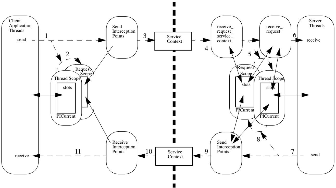
Figure 21-7 Thread Scope vs Request Scope
