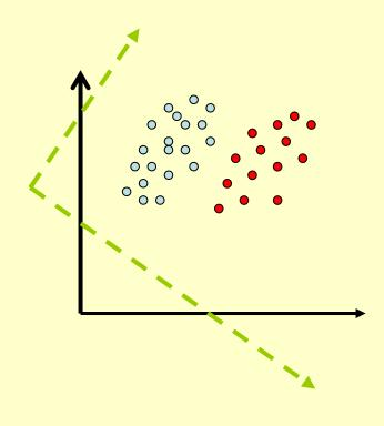
Basic idea: detect the direction of the largest variance in the data, build an axis in that. Build the other axis as orthogonal to the first axis
