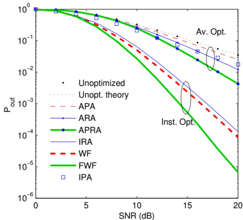
Figure:  $2 \times 2$  V-BLAST in i.i.d. Rayleigh fading channel at  $R = 3$  [nat/s/Hz]
