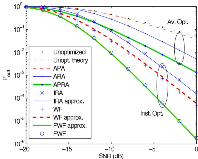
Figure:  $2 \times 2$  V-BLAST in i.i.d. Rayleigh fading channel at  $R = 0.1$  [nat/s/Hz]
