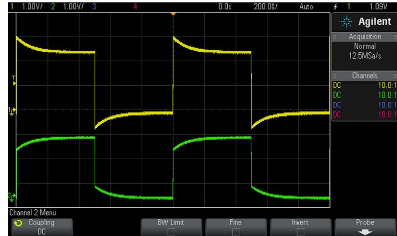
Channel-1 (yellow) = Over compensated Channel-2 (green) = Under compensated
