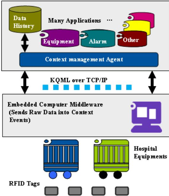
Fig. 4. Module components of the RFID system
