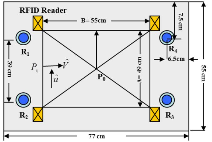
Fig. 5. Illustrated map for the size and dimensions of a mobile object with mounted RFID readers
