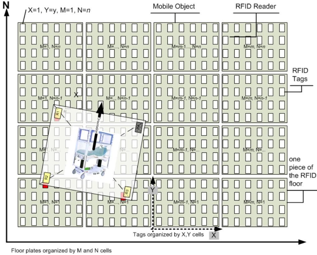
Fig. 3. An extensible RFID floor composed of  $n*m$  components with a hospital be on it
