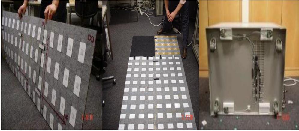
Fig. 6. The floor with RFID tags (left, middle) and mobile object with RFID readers simulating a hospital bed (right)
