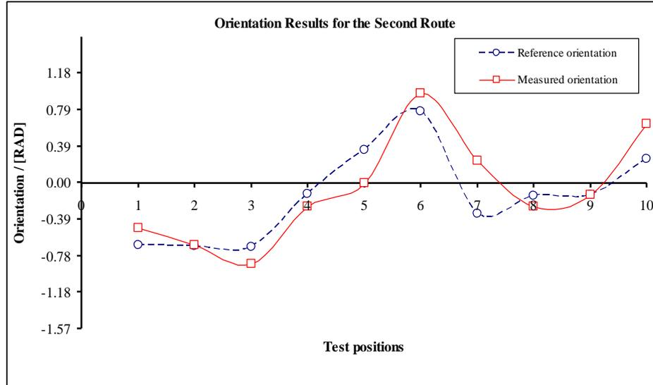
Fig. 8. Second route: Comparison of the real orientation angle with the measured angles in radian
