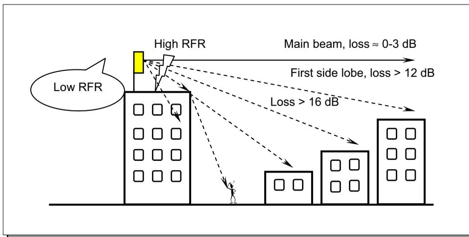
**FIGURE 1.** Conditions of RFR around a BTS.
