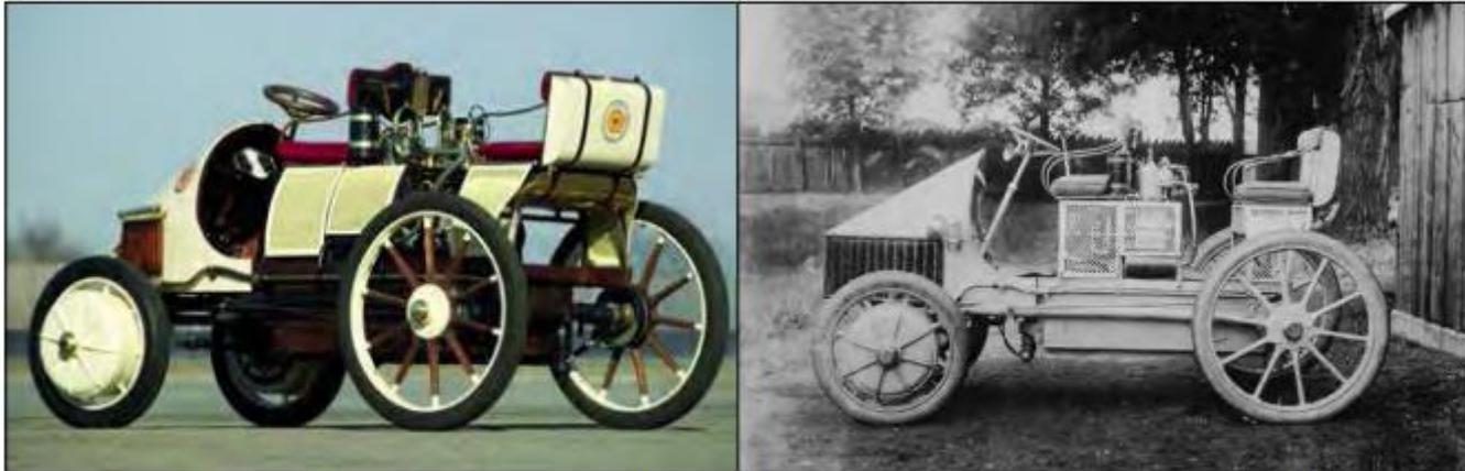
**Figure 1.** *Semper Vivus*, a Lohner-Porsche hybrid electric vehicle (right) with front in-wheel motors, which was presented at the Paris World Exhibition in 1900. **Right:** original. **Left:** a modern recreation. Photo: Porsche Cars North America
