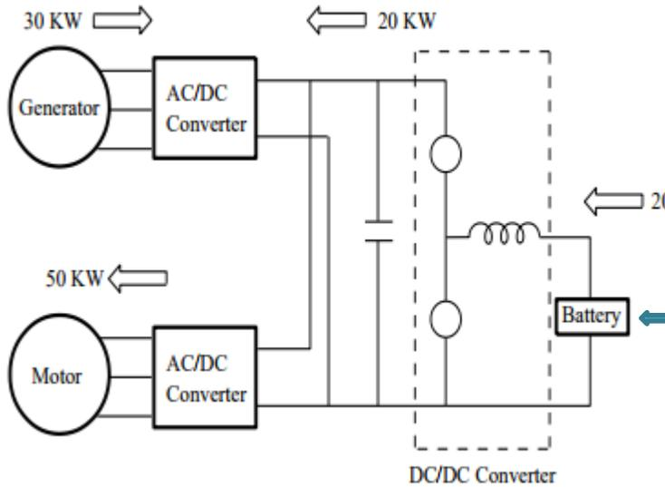
**Motor:** PMSM; 500 V; 50 kW; 8 poles, 6000 rpm
