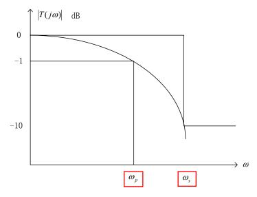
An R-C low-pass filter can be plotted as
