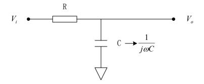
The voltage transfer function  $T(j\omega)$  is then
