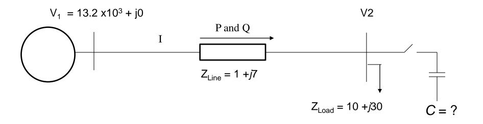
Calculate the voltage at the receiving end of the line. If the voltage is too low, compute the size of the capacitor which will recover the voltage to the same value of the sending end. Calculate the value of C.
