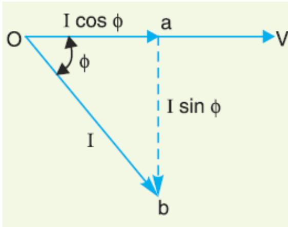
The circuit current  $I$  can be resolved into two perpendicular components, namely;
