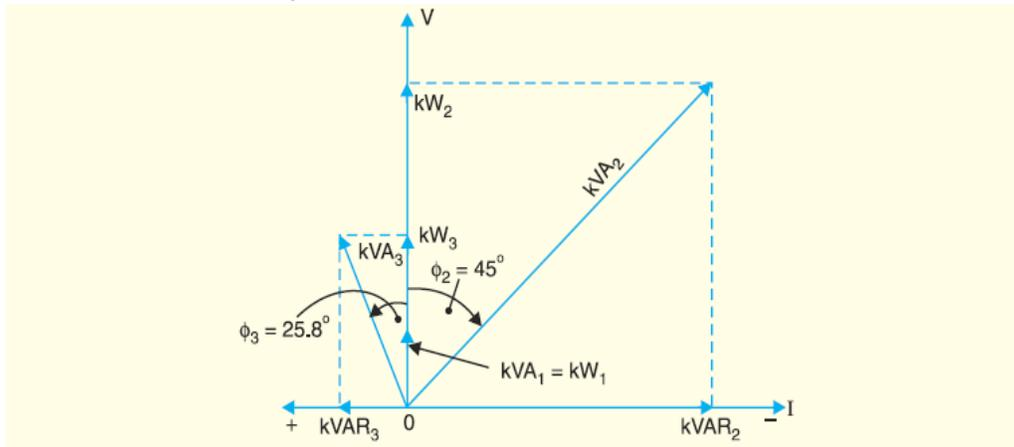
$$\text{kVAR}_1 = \text{kVA}_1 \sin \phi_1 = 20 \times 0 = 0$$
