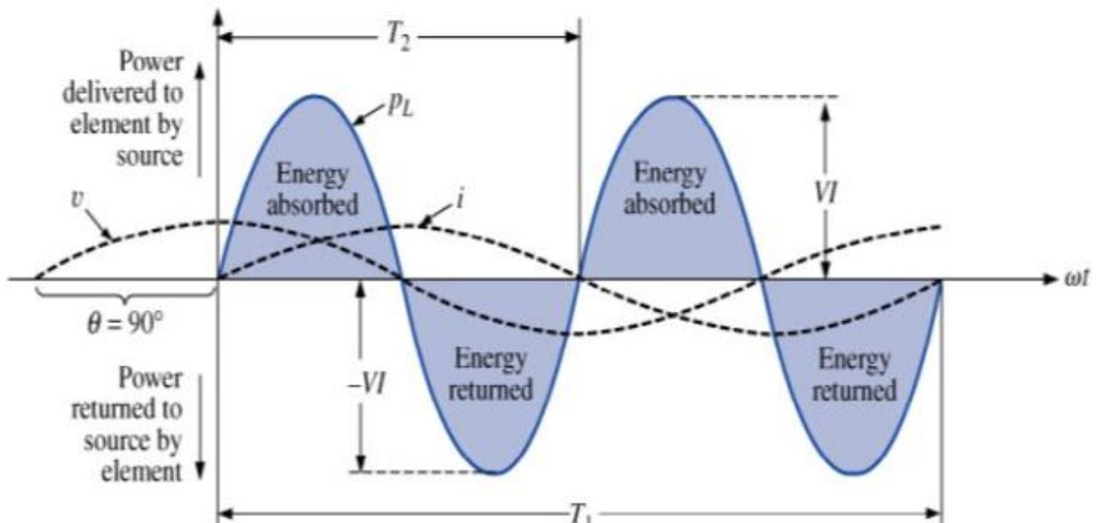
**Active power:** The active power is consumed by the active elements from a circuit (Resistances), its unit measure being the watt (W).
