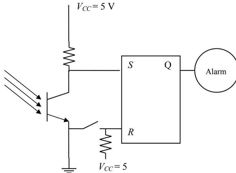
*SR* (set-rest) flip flop is constructed by NOR gates
