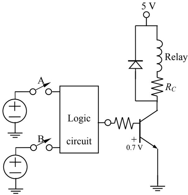
**Figure 2** Realization of a remote door lock.
