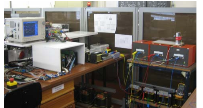
Fig. 2. Laboratory prototype of the Shunt Active Filter.
