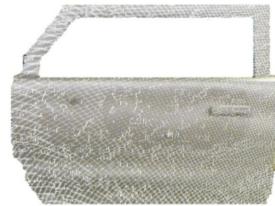
Figure 5. Triangular mesh of a door panel obtained with an accelerated meshing method.
