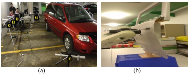
Figure 11 : Experimental setup: a) capturing 3D data over a network of Kinect sensors, and b) robot performance evaluation at following a door panel's curved surface while matching its position and orientation.
