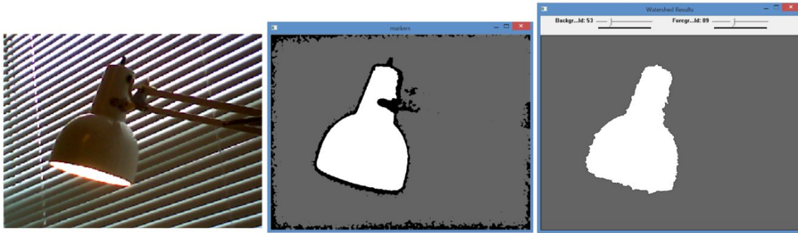
Figure 9. Improved segmentation using adjusted thresholds. Original visual image (left), thermal markers (middle) and Watershed with Thermal Markers segmentation results (right)
