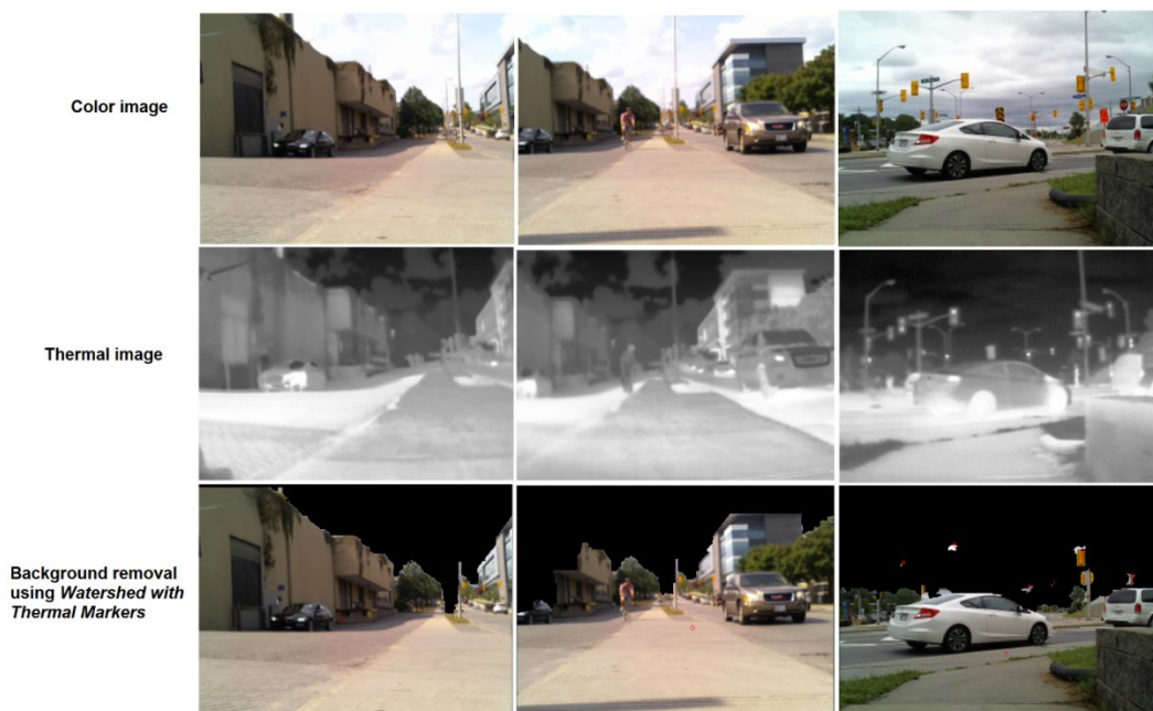
Figure 13. Watershed with Thermal Markers segmentation example to remove sky and backgrounds
