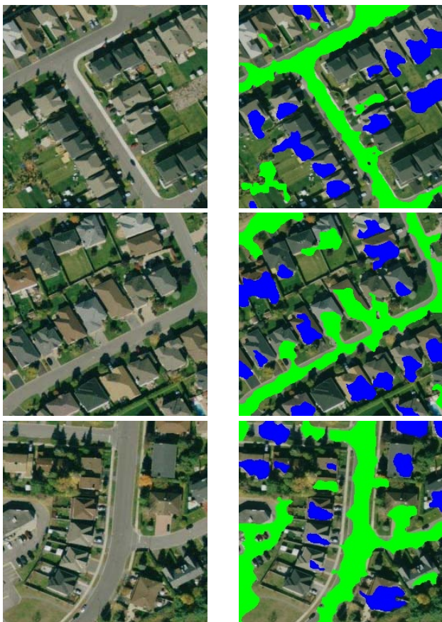
Figure 6. Left column shows some test images reproduced from Fig. 4. Right column shows the resulting labeled images. Green and blue colors represent streets and houses respectively.
