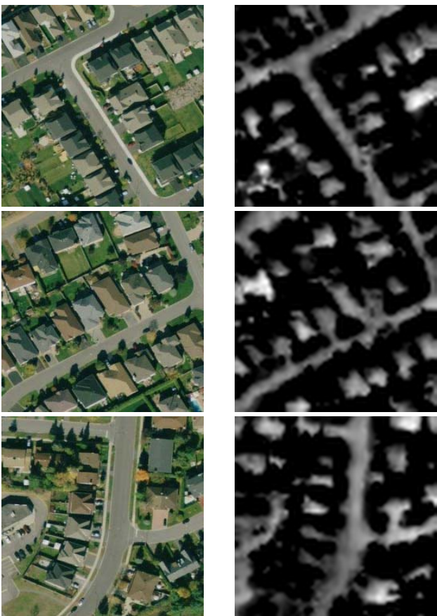
Figure 4. Test images (which were not used in the training set) are shown on the left column and corresponding top-down maps on the right. The proposed technique was able to identify most of the objects of interest. For the training set used, important objects are houses and streets.
