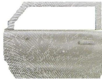
Figure 8. Triangle mesh of a car door model.
