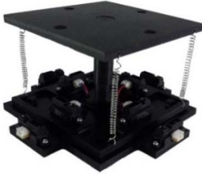
Fig.5. Prototype of the instrumented compliant wrist.
