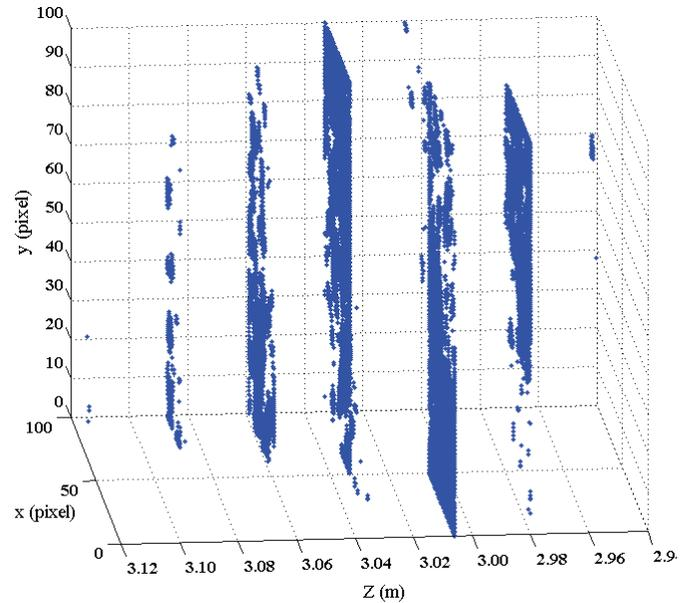
Fig. 7. Distribution of depth values of Kinect for Xbox 360 over a plane at 3m.
