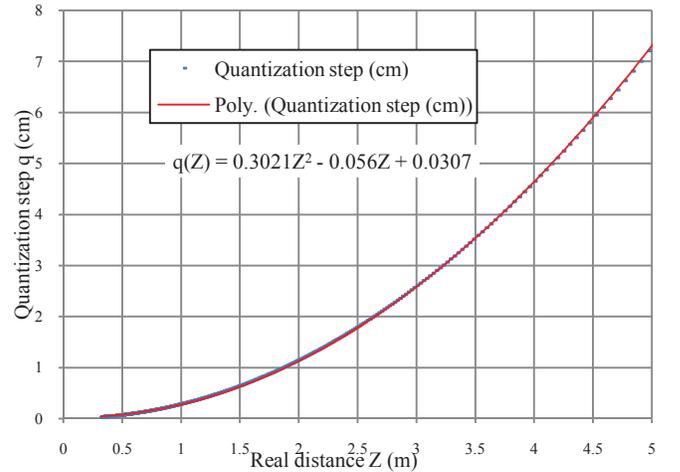
Fig. 4. Quantization step size for various distances and best quadratic curve fit.
