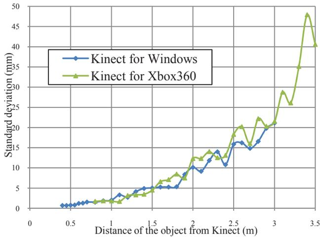
Fig. 9. Standard deviation of depth with distance.
