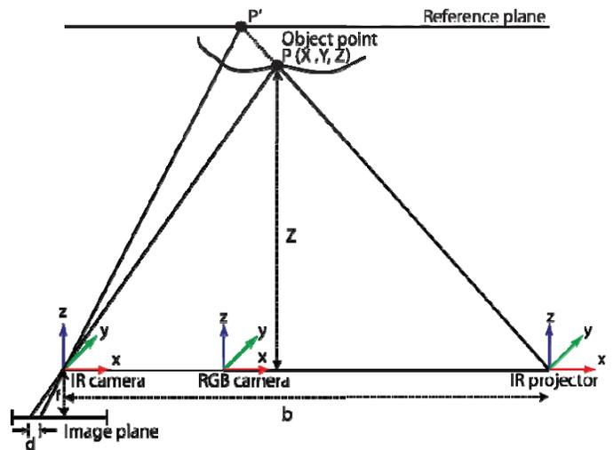
Fig. 2. Depth and disparity relationship used for depth estimation.
