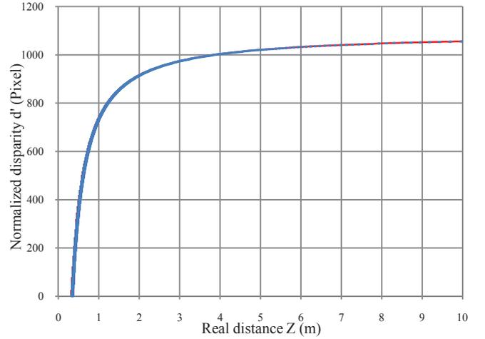
Fig. 3. Kinect normalized disparity for various distances.
