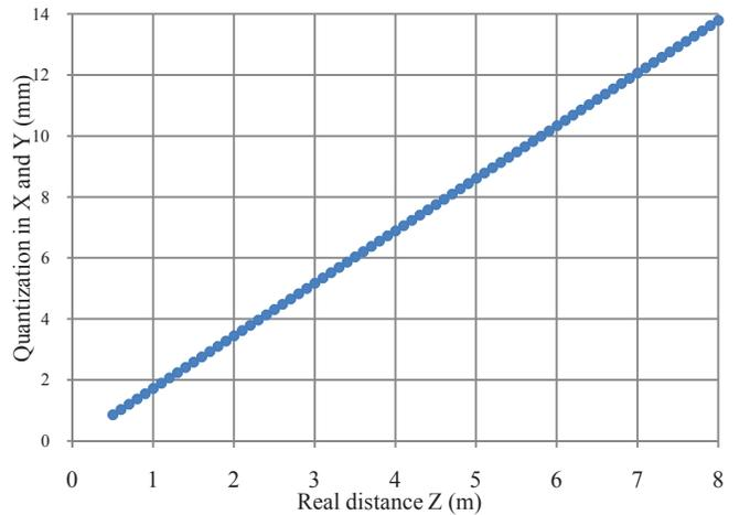
Fig. 5. Quantization step size in X and Y for various distances.
