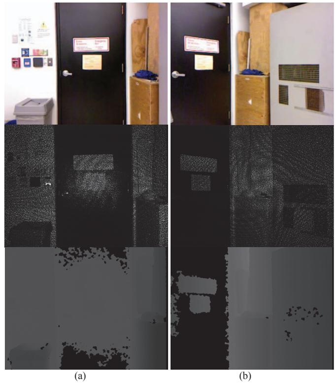
Fig. 10. Color response of Kinect depth camera on a black door. (a) Color, IR and depth images respectively, when Kinect is aligned parallel to the door, (b) Color, IR and depth images respectively, when Kinect's pose is modified.
