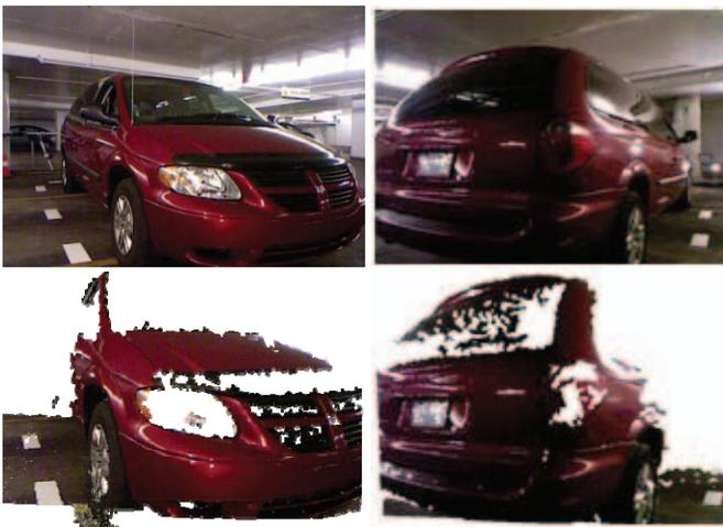
Fig. 12. Two views of a vehicle (top) and corresponding 3D reconstructions (bottom), with missing depth areas depicted in white.
