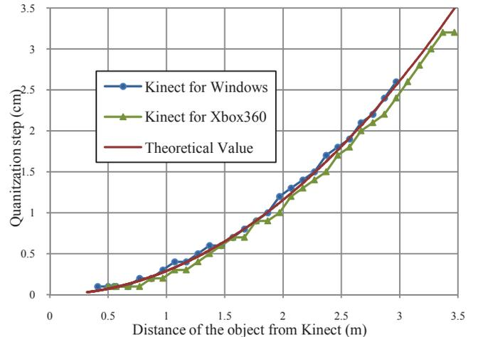
Fig. 8. Experimental quantization step size as a function of distance.
