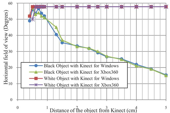
Fig. 11. Response of the Kinect sensor over surfaces with different colors and reflectance characteristics. Angles show the effective area seen by the depth sensor.
