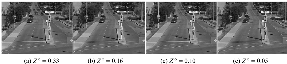
Fig. 4. Effect of threshold value Z^o on the moving pixels elimination from background model - lower Z^o benefits in completeness of the operation: (a) 0.33; (b) 0.16; (c) 0.10 and (d) 0.05.
