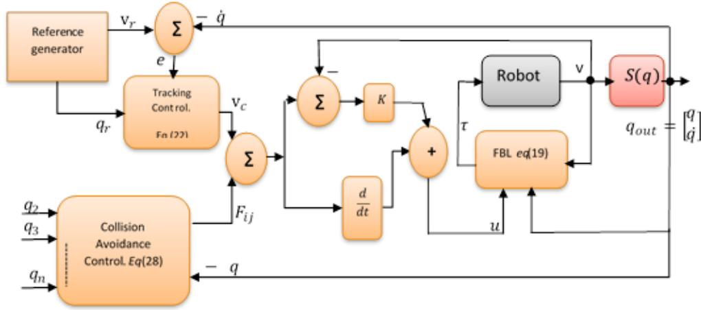
Figure 2. Schematic diagram of the proposed formation controller.
