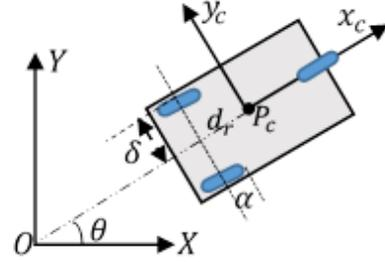
Figure 1. A nonholonomic mobile robot internal Cartesian frame.
