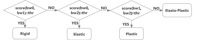
Fig. 6. Classification process for rigid, elastic, plastic, and elasto-plastic materials.
