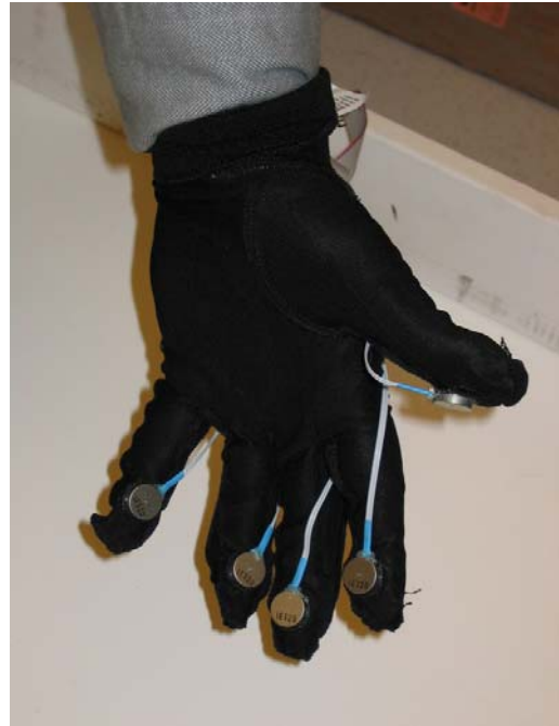
Figure 13. Tactile fingertip human interface.
