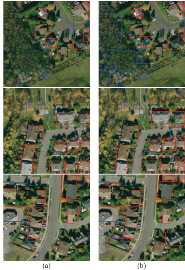
Figure 5. Detected buildings, shown in red, and detected streets and distractors, shown in blue for (a) simple watershed, (b) recursive watershed.
