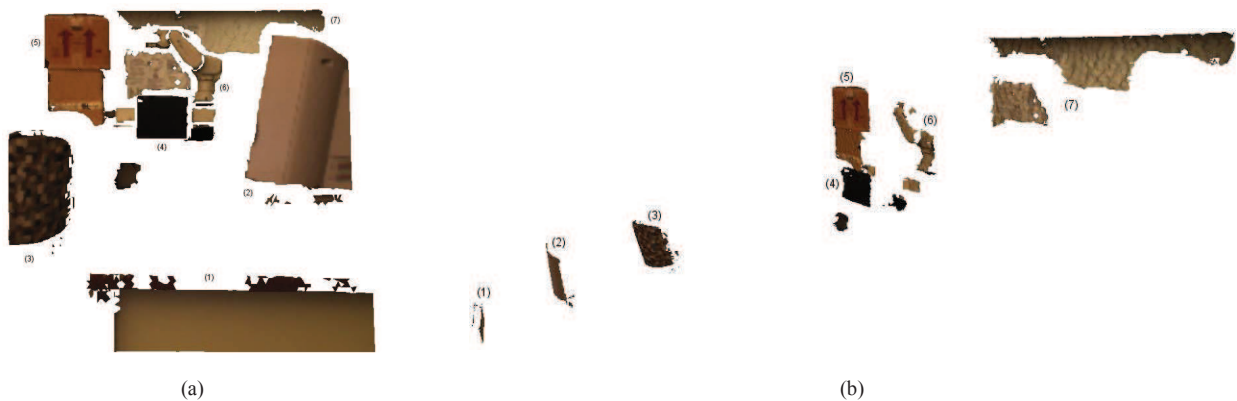
Fig. 8. (a) Reconstructed scene from the sensor's viewpoint, and (b) same reconstruction from a side view showing the depth of field.
