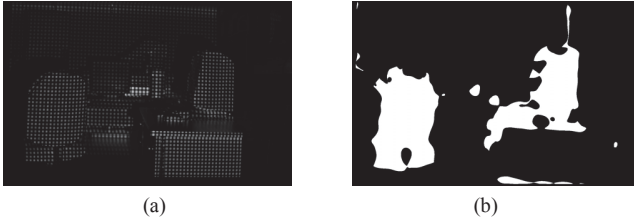
Fig. 4. (a) Example of an image collected from one focus plane where closer objects are in focus, and (b) its corresponding sharpness mask.
