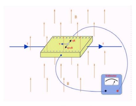
Figure 1: A schematics of the experimental setup of the Hall effect. A current driven through the conductor, drawn as a prism, leads to the emergence of voltage in the perpendicular direction. This is the Hall voltage, which Maxwell erroneously predicted to be zero.
