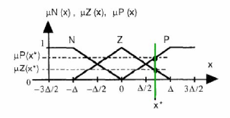
Membership functions and the quantization characteristics for a 3-set (N, Z, and P) fuzzy partition of the domain where the analog variable x is defined. XFQ are the crisp analog values recovered after a defuzzification of the fuzzy converted value x. It also shows the truncated information XQ recovered from an A/D converter with 3 quantization levels ("-1", "0", and "+1) defined over the same domain for x.
