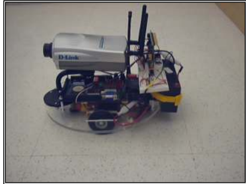
Two-wheel robotic platform for an experimental mobile autonomous robotic sensor agent equipped with a wireless camera, IR sensors and on computational power
