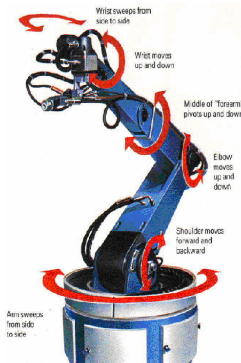
Motions of an articulated robot arm.
