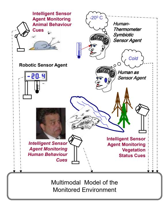
Heterogeneous network of robotic sensors, human-transducer symbiotic sensor agents, human sensor agents, and *intelligent sensor agents capable to comprehend human and animal behaviour, and vegetation status.*  *Symbionts* combine intrinsic machine-sensing reactive behavior with higher-order human-oriented world-model representations of the immersive virtual reality.
