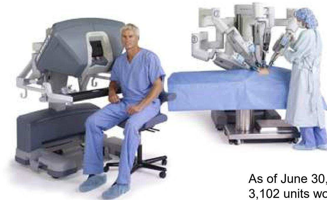
*Da Vinci System* allows the surgeon's hand movements to be translated into smaller, precise movements of tiny instruments inside the patient's body.
